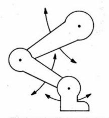
This is a simplified sketch, but it shows that only three moves are required to make the leg functional. Each section of the leg can be treated as "Lever B" in the double windlass mechanism described here. Each section can be powered and controlled individually, drawing power from the single main motor.
