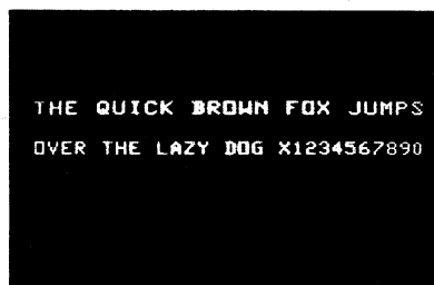
Figure 10b. Example of Character Generation Using Pedestal-type Scan.
