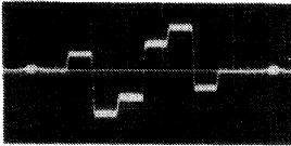
Fig. 21(d) - CA3072 - terminal No. 11, 5.2 v p-p R-Y output, one horizontal line
