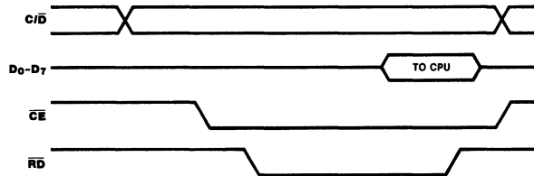
Figure 9. Non-Z-BUS Read Cycle Timing
