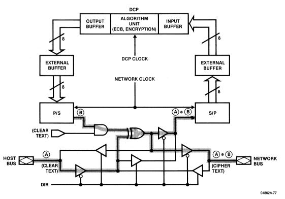
Figure 4.45. Bidirectional Interface, Transmit Mode
