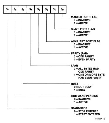
Figure 3.5. Status Register Bit Assignments
