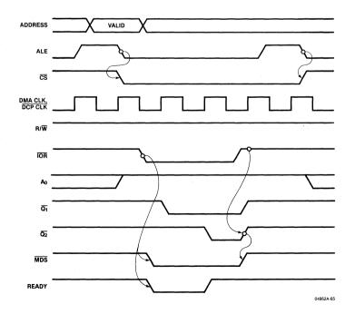
Figure 4.33. Data Read Cycle Timing
