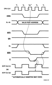
Figure 4.23. Data Read Cycle (Mode B)
