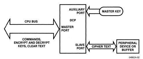
Figure 2.7. Data Flow for Dual Port Configuration, Multiplexed Control Mode
