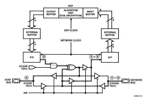
Figure 4.46. Bidirectional Interface, Receive Mode
