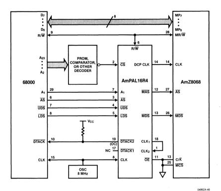
Figure 4.14. AmZ8068 to 68000 Connection Using a PAL
