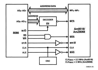
Figure 4.4. Direct Interface 8086-Am9518/AmZ8068 (Minimum Mode)
