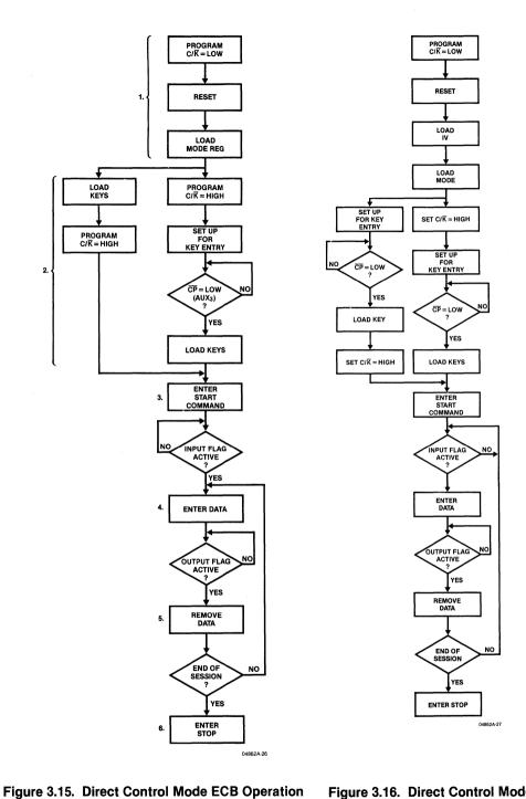
Figure 3.16. Direct Control Mode CBC/CFB Operation
