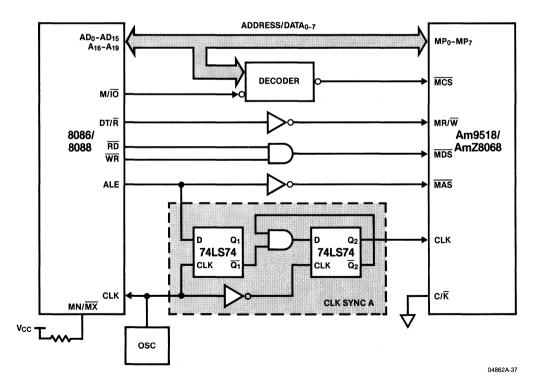
Figure 4.5. 8086/8088-Am9518/AmZ8068 Interface (Minimum Mode)
