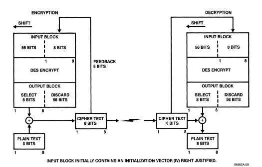
Figure 2.3. 8-Bit Cipher Feedback (CFB) Mode
