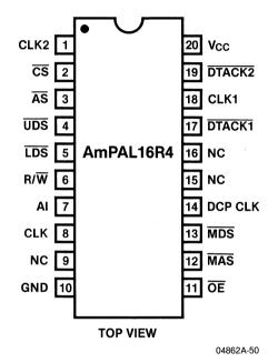
Figure 4.18. AmPAL16R4 Connection Diagram
