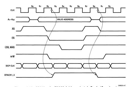
Figure 4.15. 68000—AmZ8068 Address Latch Cycle ( $A_1 = Low$ )
