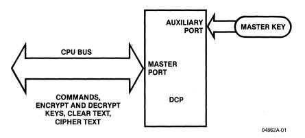
Figure 2.6. Data Flow for Single Port Configuration, Multiplexed Control Mode
