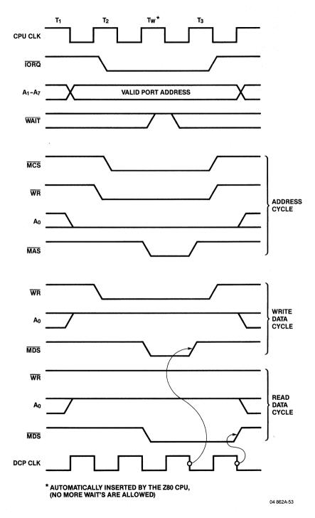
Figure 4.21. Z80-Am9518/Z80A-AmZ8068 Timing Diagram (Mode A)
