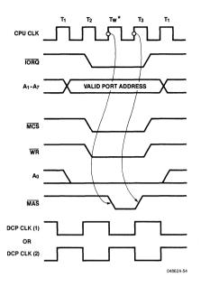
Figure 4.22. Address Latch Cycle (Mode B) (No Clock Synchronization)
