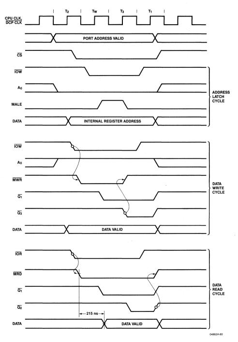
Figure 4.28. CPU-DCP Timing Diagram
