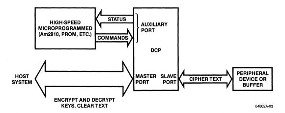
Figure 2.8. Data Flow for Dual Port Configuration, Direct Control Mode
