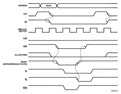
Figure 4.31. Address Latch Cycle Timing (CPU-DCP)
