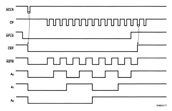
Figure 4.39. Auxiliary Port Key Load Timing
