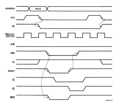
Figure 4.32. Data Write Cycle Timing (CPU-DCP)
