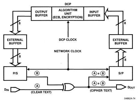
Figure 4.42. Network Transmitter
