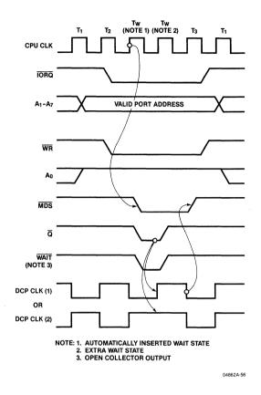
Figure 4.24. Data Write Cycle (Mode B)
