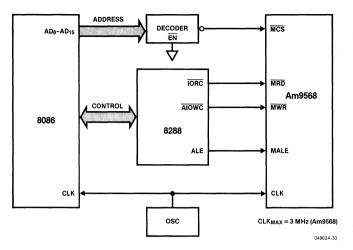
Figure 4.1. Direct Interface 8086-Am9568 (Maximum Mode)
