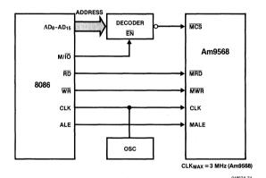
Figure 4.2. Direct Interface 8086-Am9568 (Minimum Mode)
