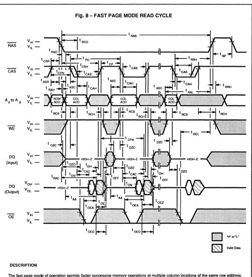
The fast page mode of operation permits faster successive memory operations at multiple column locations of the same row address. This operation is performed by strobing in the row address and maintaining RAS at a Low level and WE at a High level during all successive memory cycles in which the row address is latched. The access time is determined by tCAC, tAA, tCPA, or tOEA, which ever one is the latest in occuring.
