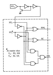
Fig. 16-Master slice/wire bond option control circuitry.
