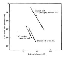
Fig. 9-Comparison of SER for three types of cell structure.
