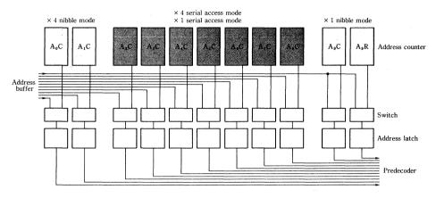
Fig. 17-Address counter block diagram for nibble mode and serial access mode.
