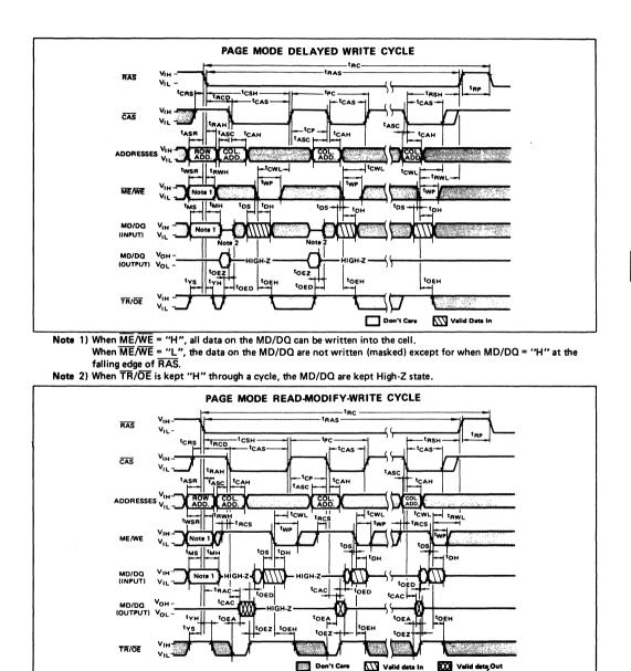
Note 1) When ME/WE = "H", all data on the MD/DQ can be written into the cell. When ME/WE = "L", the data on the MD/DQ are not written (masked) except for when MD/DQ = "H" at the falling edge of RAS.
