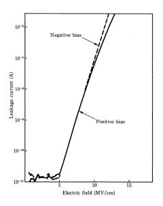
Fig. 14-Leakage current of capacitor film.
