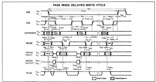
Note 1) When ME/WE = "H", all data on the MD/DQ can be written into the cell. When ME/WE = "L", the data on the MD/DQ are not written (masked) except for when MD/DQ = "H" at the falling edge of RAS.
