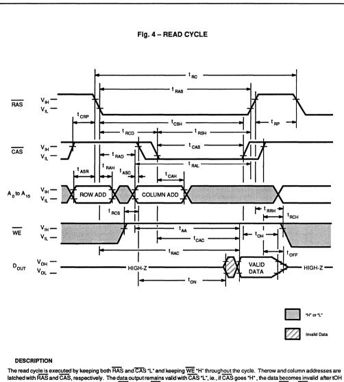
Ine read cycle is executed by keeping both RAS and CAS \*L and keeping weer in throughout the cycle. Therow and column addresses are latched with RAS and CAS, respectively. The data output remains valid with CAS \*L\*, ie., if CAS goes \*H\*, the data becomes invalid after tOH is satisfied. The access time is determined by RAS (tRAC), CAS (tCAC), or Column address input (tAA). If tRCD (RAS to CAS delay time) is greater than the specification, the access time is tAA.
