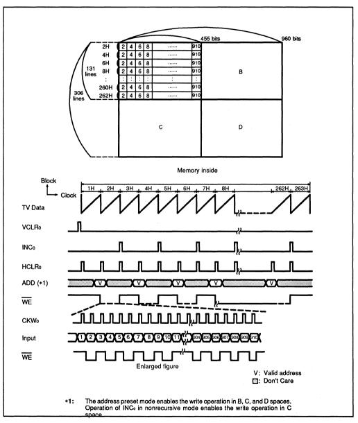
3. Write operation of 1/2 compressed data to memory: In nonrecursive mode, address preset mode
