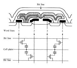
Fig. 7-3D stacked capacitor cell.
