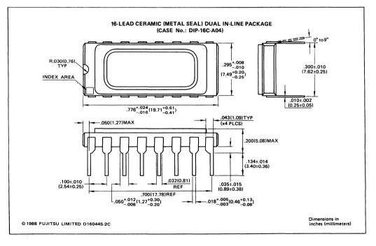
Standard 16-pin Ceramic DIP (Suffix: -Z)
