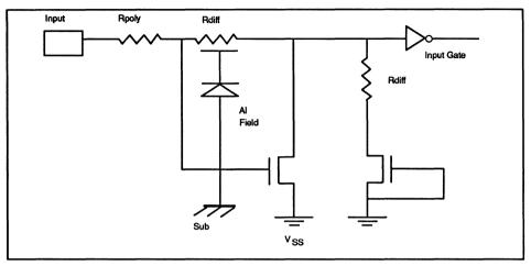
Figure 4. 1-megabit CMOS DRAM Input Protection Circuit
