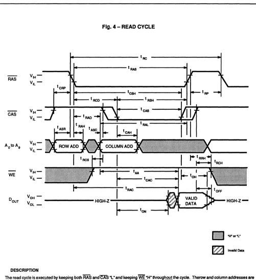
The read cycle is executed by keeping both FAS and CAS "L" and keeping <u>WE</u>"H" throughout the cycle. I herow and column addresses are latched with RAS and CAS, respectively. The data output remains valid with CAS "L", i.e., if CAS goes "H", the data <u>becomes invalid</u> after tOH is satisfied. The access time is determined by RAS (IRAC), CAS (ICAC), or Column address input (IAA). If IRCD (RAS to CAS delay time) is greater than the specification, the access time is IAA.
