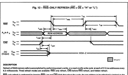
RAS-only refresh is performed by keeping RAS Low and CAS High throughout the cycle; the row address to be refreshed is latched on the falling edge of RAS. During RAS-only refresh, Dout pin is kept in a high-impedance state.
