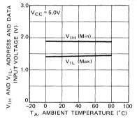
Fig. 19 – RAS, CAS, WE AND OE INPUT VOLTAGE vs. AMBIENT TEMPERATURE
