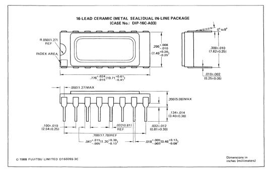
Standard 16-pin Ceramic DIP (Suffix: -C)
