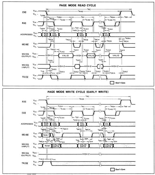
Note 1) When  $\overline{ME}/\overline{WE}$  = "H", all data on the MD/DQ can be written into the cell.
