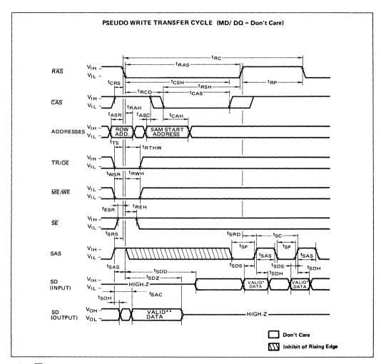
\*: If  $\overline{SE}$  is high, these data are not written into SAM. \*\*: If  $\overline{SE}$  is high, SD (SD0 to SD3) are in High-Z state after  $t_{SEZ}$ . If  $\overline{SE}$  becomes low, the valid data will appear meeting  $t_{SAC}$  and  $t_{SEA}$ .
