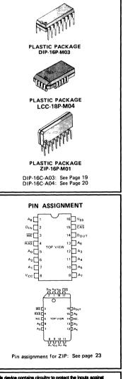
This device contains circuitry to protect the inputs against damage due to high static voltages or electric fields. However, it is advised that normal precautions be taken to avoid application of any voltage higher than maximum rated voltages to this high impedance circuit.
