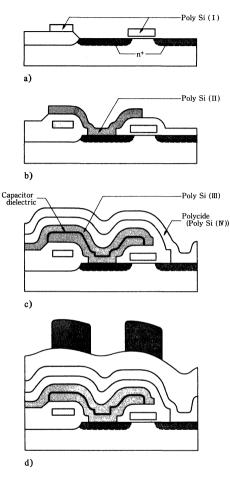
Fig. 12-Schematic veiw of 3D stacked capacitor cell and fabrication process.
