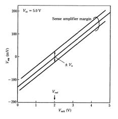
Fig. 6-Relation between  $V_{cell}$  and  $V_{sig}$  (Dummy cell is adjusted to fit  $V_{ref} = 2 V$ ).
