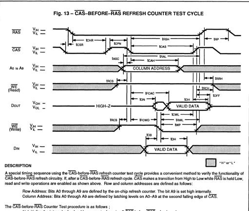
1) Initialize the internal refresh address counter by using 8 CAS-before-RAS refresh cycles.
