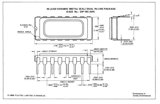
Standard 16-pin Ceramic DIP (Suffix: -Z)
