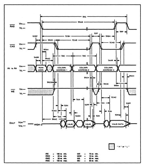
Figure 2. Typical Static Mode Read Cycle
