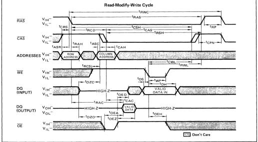
Note: 1) When  $\overline{OE}$  is kept high through a cycle, the DQ pins are kept high-Z state.
