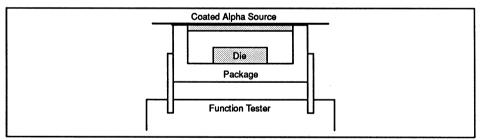
Figure 3. Alpha Source Acceleration Test
