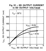
Fig. 33 – SD OUTPUT CURRENT vs SD OUTPUT VOLTAGE
