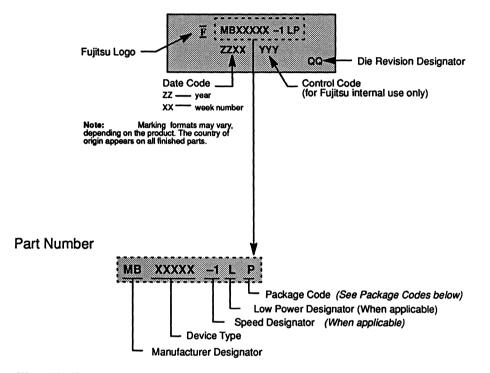
MB Identifies an IC designed and manufactured by Fujitsu with a Fujitsu-designated device number.
