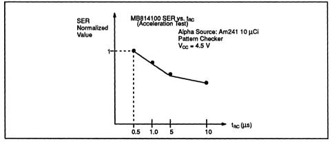
Figue 5. Soft Error Rate vs. t<sub>RC</sub> (MB814100)
