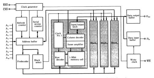
Fig. 20-Block diagram of 4M DRAM (Address clocks shape whole chip, but each 1-Mbit blocks has its own clock generator).
