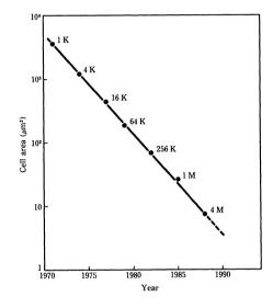
Fig. 2-History of cell area reduction (Cell area reduced by a factor of 400 in 18 years).
