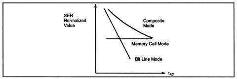
Figure 2. Soft Error Rate vs. Cycle Time
