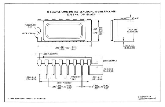
Standard 16-pin Ceramic DIP (Suffix: -C)
