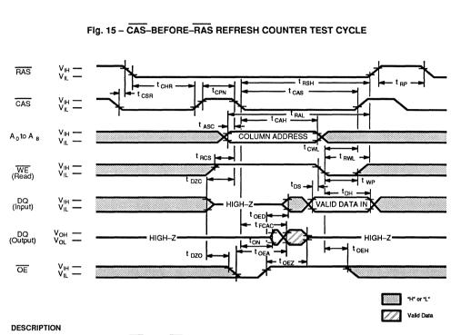
A special timing sequence using the CAS-before-RAS refresh counter test cycle provides a convenient method to verify the functionality of CAS-before-RAS refresh circuitry. If, after a CAS-before-RAS refresh cycle. CAS makes a transition from High to Low while RAS is held Low, read and write operations are enabled as shown above. Row and column addresses are defined as follows:
