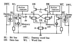
Fig. 4-Sense amplifier circuitry of 254-K DRAM.
