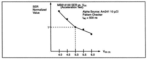
Figure 4. Soft Error Rate vs. V<sub>CC</sub> (MB814100)
