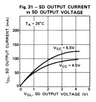
Fig. 33 – SD OUTPUT CURRENT vs SD OUTPUT VOLTAGE
