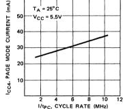
Fig. 17 - REFRESH CURRENT 2 vs CYCLE RATE
