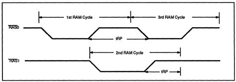
Figure 10. RAS Timing of Interleaving Memory
