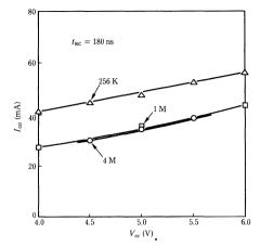
Fig. 23-Average  $V_{cc}$  current ( $I_{ccl}$ ) vs  $V_{cc}$  voltage.
