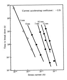
Fig. 15-Stress current on lifetime (0.1% cumulative failure).
