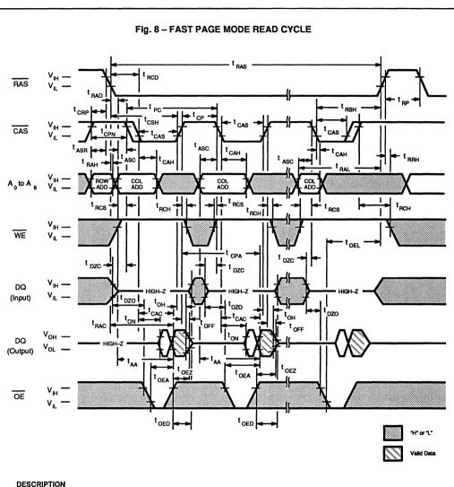
The fast page mode of operation permits faster successive memory operations at multiple column locations of the same row address. This operation is performed by strobing in the row address and maintaining RAS at a Low level and WE at a High level during all successive memory cycles in which the row address is latched. The access time is determined by tCAC, tAA, tCPA, or tOEA, whichever one is the latest in occuring.
