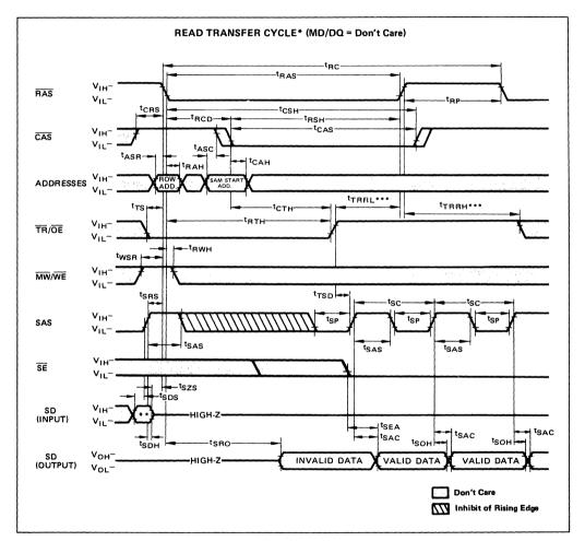
\*: In the case that the previous transfer is write transfer. \*\*; If SE is low and the previous cycle is serial write cycle, this should be valid data input. \*\*\*; These parameters are different from that of MB 81461.
