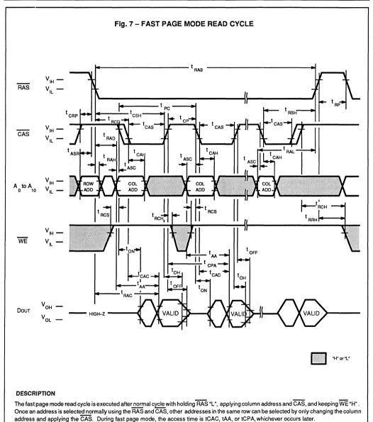
address and applying the CAS. During fast page mode, the access tin Any of the 2048 bits belonging to each row can be accessed.
