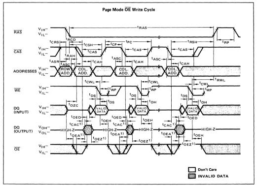
Note: 1) When  $\overline{OE}$  is kept high through a cycle, the DQ pins are kept high-Z state.
