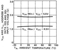
Fig. 27 – RAS, CAS, ME/WE, TR/OE, SE, SAS INPUT VOLTAGE vs AMBIENT TEMPERATURE
