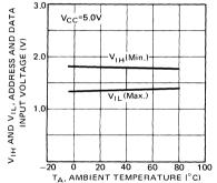
Fig. 20 – RAS, CAS AND WE INPUT VOLTAGE vs AMBIENT TEMPERATURE
