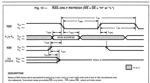
RAS-only refresh is performed by keeping RAS Low and CAS High throughout the cycle; the row address to be refreshed is latched on the tailing edge of RAS. During RAS-only refresh, DO pins are kept in a high-impedance state.
