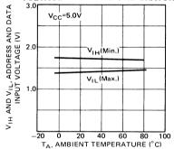
Fig. 19 –  $\overline{RAS}$ ,  $\overline{CAS}$  AND  $\overline{WE}$  INPUT VOLTAGE vs AMBIENT TEMPERATURE
