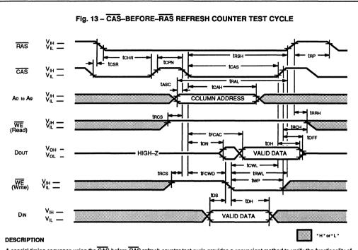
A special timing sequence using the CAS-before-RAS refresh counter test cycle provides a convenient method to verify the functionality of CAS-before-RAS refresh circuitry. If, after a CAS-before-RAS refresh cycle. CAS makes a transition from High to Low while RAS is held Low, read and write operations are enabled as shown above. Row and column addresses are defined as follows:
