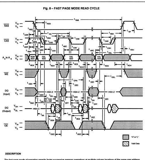
The fast page mode of operation permits faster successive memory operations at multiple column locations of the same row address. This operation is performed by strobing in the row address and maintaining  $\overline{\text{PAS}}$  at a Low level and  $\overline{\text{WE}}$  at a High level during all successive memory cycles in which the row address is latched. The access time is determined by tCAC, tAA, tCPA, or tOEA, whichever one is the latest in occuring.
