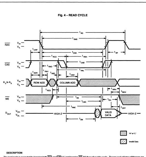
The read cycle is executed by keeping both FAS and CAS "L" and keeping WE "H" throughout the cycle. Therow and column addresses are latched with FAS and CAS, respectively. The data output remains valid with CAS "L", i.e., if CAS goes "H", the data becomes invalid after tOH is satisfied. The access time is determined by FAS (tRAC), CAS (tCAC), or Column address input (tAA). If tRCD (FAS to CAS delay time) is greater than the specification, the access time is tAA.
