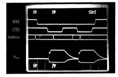
Fig. 22-Output wave form operating in a fast page mode.
