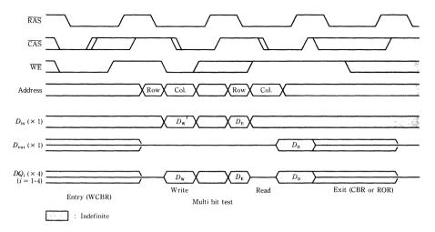
Fig. 21-Timing diagram of 16-bit multi bit test (D<sub>W</sub>, D<sub>R</sub>, D<sub>E</sub> are write, read, expected data).
