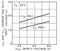
Fig. 18 – RAS, CAS, WE AND OE INPUT VOLTAGE vs. SUPPLY VOLTAGE
