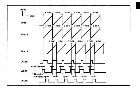
In the field memory (three ports) is used, stable output can be obtained, regardless of jitter from the write clock. In addition, the correlation between frames or lines can be calculated.
