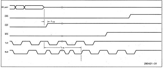
Figure 32. TPE Collision Timings (End of Collision)
