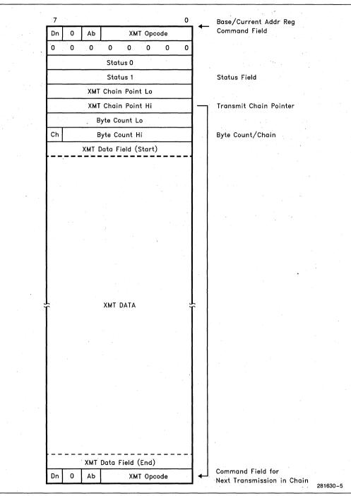
Figure 7-2. XMT Block Memory Structure (8-Bit)
