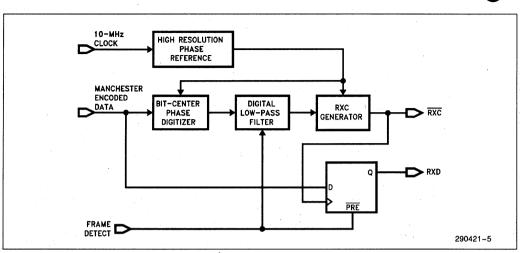
Figure 6. Manchester Decoder and Clock Recovery
