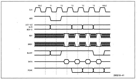
Figure 45. Basic 82596CA Burst Cycle
