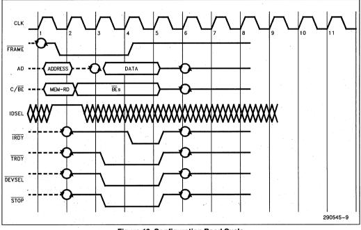
Figure 10. Configuration Read Cycle
