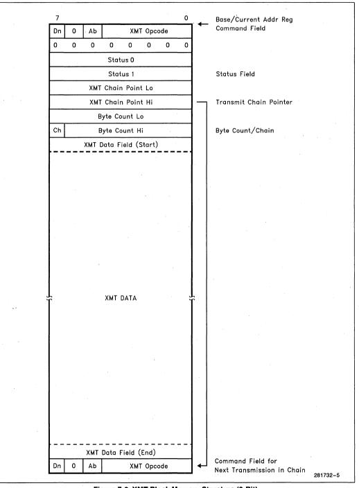
Figure 7-2. XMT Block Memory Structure (8-Bit)
