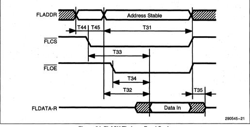
Figure 24. FLASH Timings: Read Cycle
