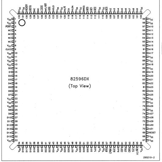
Figure 2a. 82596DX PQFP Pin Configuration
