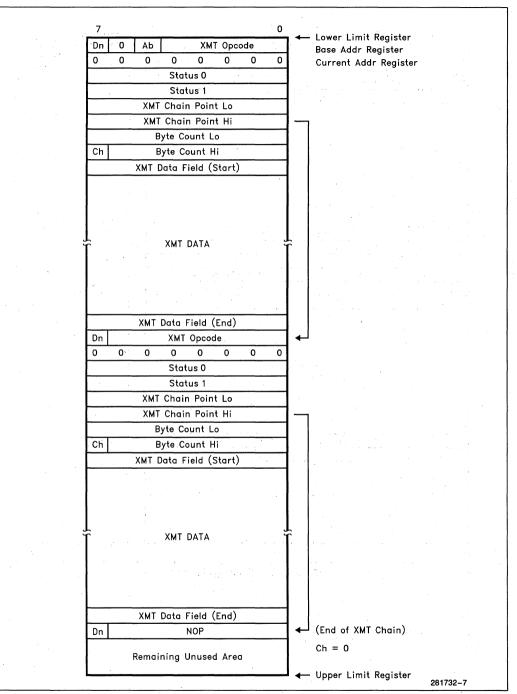
Figure 7-5. XMT Block Memory Structure (8-Bit)
