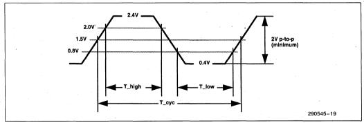
Figure 21. Clock Waveform
