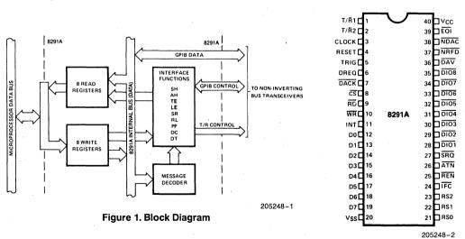
Figure 2. Pin Configuration
