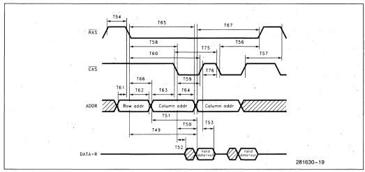
Figure 11-9. DRAM Timing Diagram: Fast Page Mode—Read Cycle
