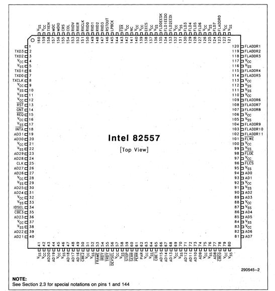
Figure 2. Device Pinout, Top View
