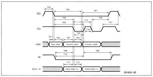
Figure 11-10. DRAM Timing Diagrams: Fast Page Mode—Write Cycle
