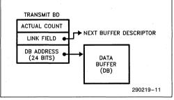
Figure 11. Data Buffer Descriptor and Data Buffer Structure
