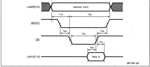
Figure 11-10. FLASH Timings—Write Cycle
