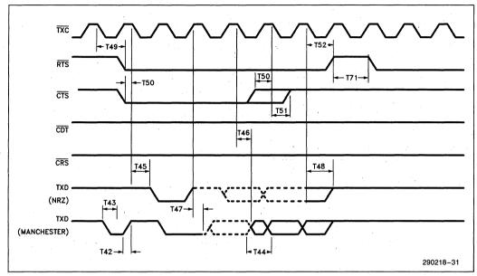
Figure 58. Transmit Data Waveforms
