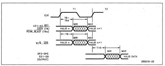
Figure 52. Output Valid Delay Timing
