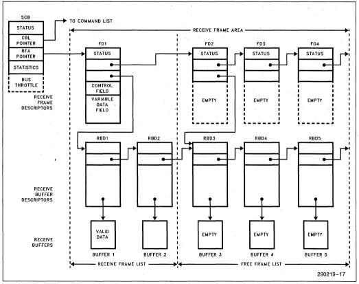
Figure 39. RFA Flexible Memory Structure
