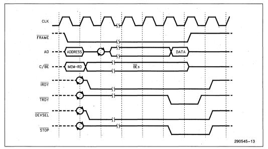
Figure 14. Flash Buffer Read Cycles
