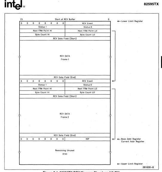
Figure 8-1. 82595TX RCV Memory Structure (16-Bit)
