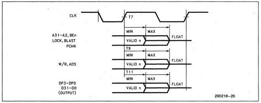
Figure 53. Output Float Delay Timing
