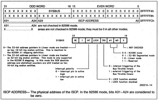
Figure 15. The System Configuration Pointer
