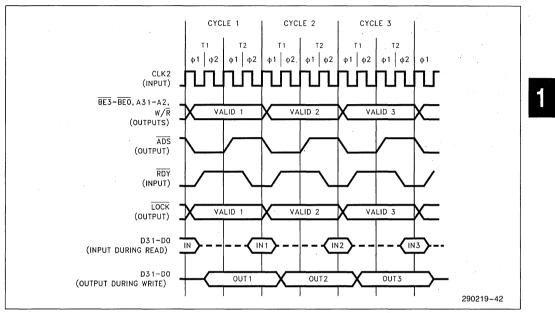
Figure 44. Basic 82596DX Bus Cycles
