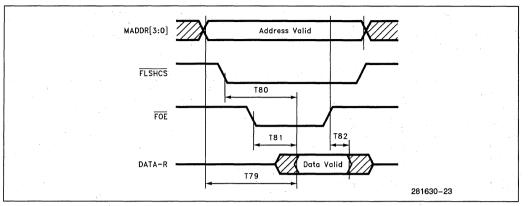
Figure 11-13. Flash Timings—Read Cycle
