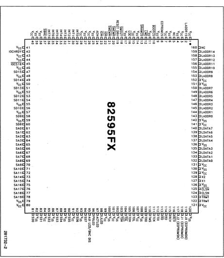
Figure 2. 82595FX Pinout
