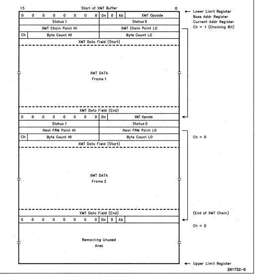
Figure 7-4. 82595FX XMT Chaining Memory Structure
