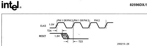
Figure 55. RESET Input Timing
