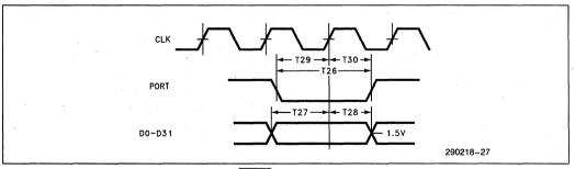
Figure 54. PORT Setup and Hold Time
