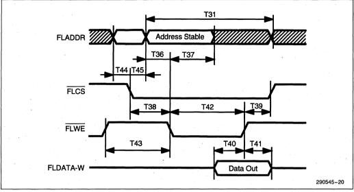
Figure 23. FLASH Timings: Write Cycle
