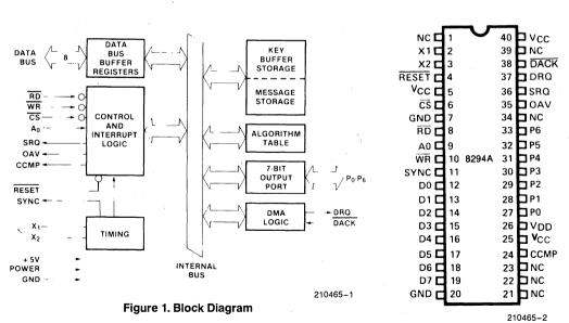
Figure 2. Pin Configuration
