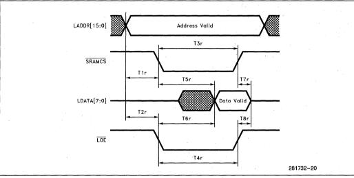
Figure 11-8. SRAM Timings—Read Cycle
