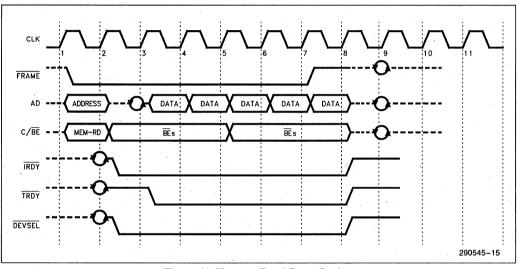
Figure 16. Memory Read Burst Cycles
