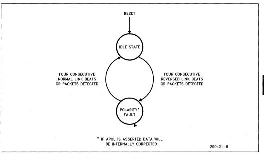
Figure 7. Polarity Fault State Diagram
