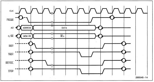
Figure 15. Flash Buffer Write Cycle
