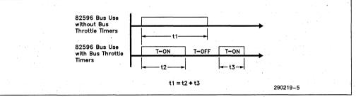
Figure 5. Bus Throttle Timers
