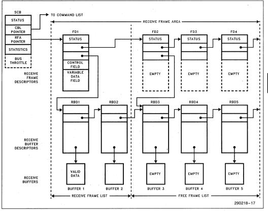
Figure 39. RFA Flexible Memory Structure
