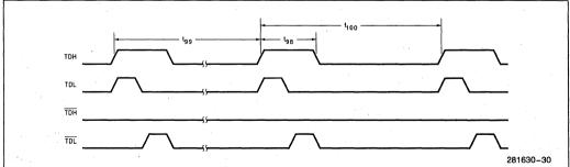
Figure 11-19. TPE Transmit Timings (Link Test Pulse)
