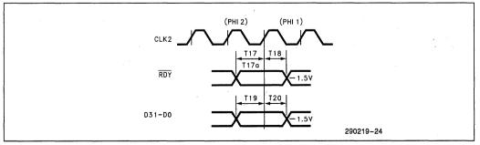
Figure 51. Input Setup and Hold Time
