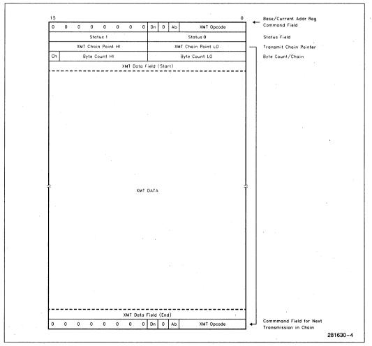
Figure 7-1. XMT Block Memory Structure (16-Bit)
