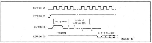
Figure 18. 82557 EEPROM Timing Diagram (Example Read from Address 0)
