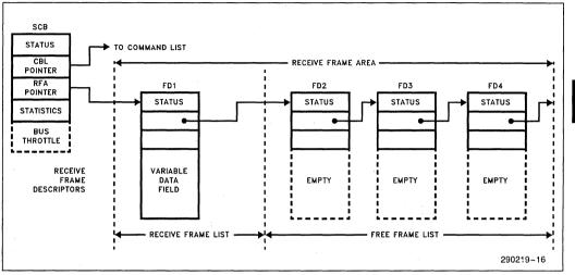
Figure 38. RFA Simplified Memory Structure
