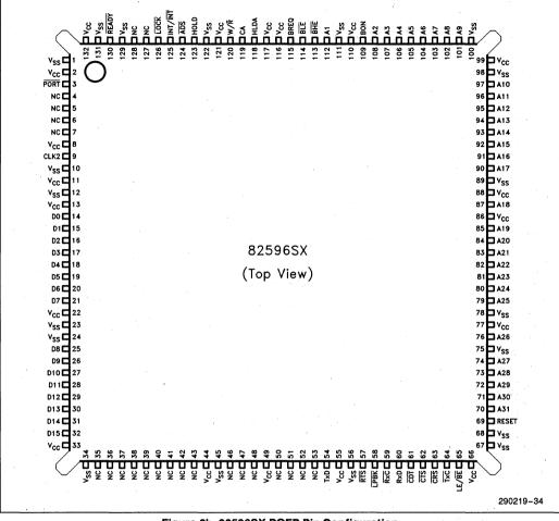
Figure 2b. 82596SX PQFP Pin Configuration
