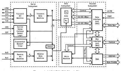
Figure 1. 82596DX/SX Block Diagram
