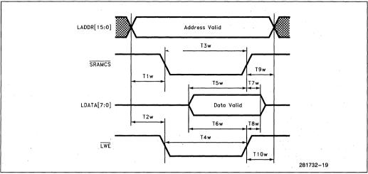
Figure 11-7. SRAM Timings—Write Cycle
