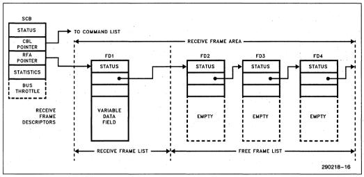
Figure 38. RFA Simplified Memory Structure
