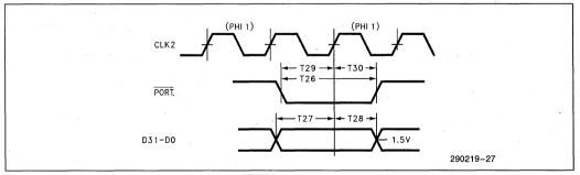
Figure 54. PORT Setup and Hold Time
