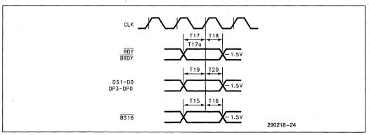
Figure 51. Input Setup and Hold Time
