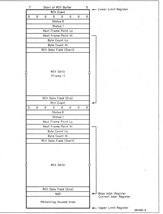
Figure 8-2. 82595TX RCV Memory Structure (8-Bit)
