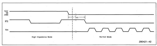
Figure 44. Reset Timings (End of Low Power Mode)
