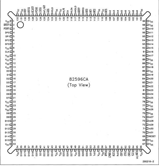
Figure 2. 82596CA PQFP Pin Configuration
