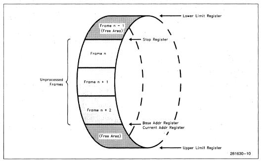
Figure 8-4. 82595TX RCV Ring Buffer Operation
