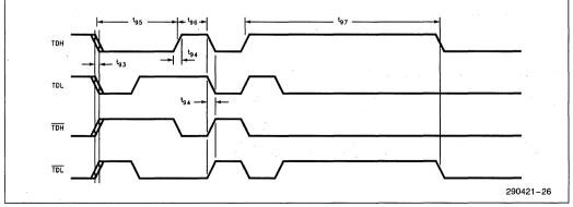
Figure 27. TPE Transmit Timings (End of Frame)
