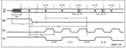
Figure 29. TPE Receive Timings (Start of Frame)
