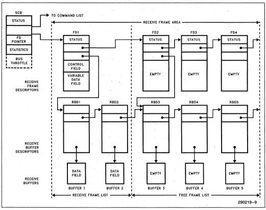
Figure 9. Flexible Memory Structure
