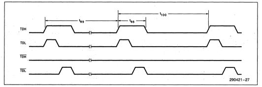
Figure 28. TPE Transmit Timings (Link Test Pulse)
