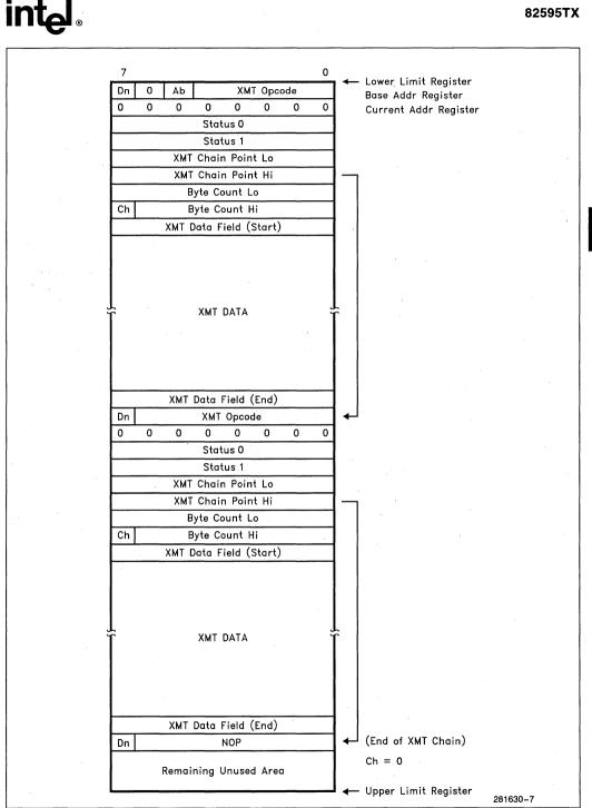
Figure 7-5. XMT Block Memory Structure (8-Bit)
