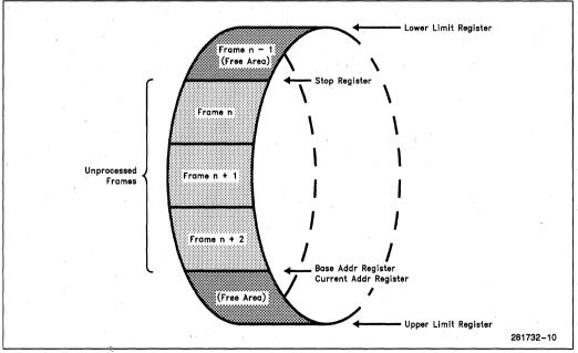
Figure 8-4. 82595FX RCV Ring Buffer Operation
