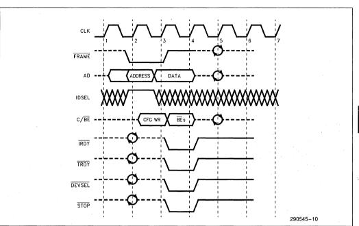
Figure 11. Configuration Write Cycle
