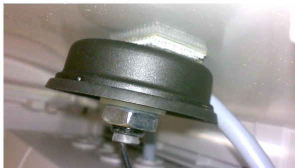
Fig. 75: Mounting UMTS antenna
