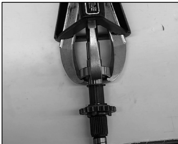
17. Remove bearing from other end of input shaft. Remove two snap rings and gear.
