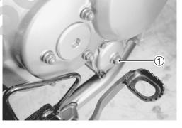
Install the oil pressure gauge and adaptor into the main oil gallery.
