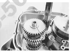
Reassemble the shift cam lock shaft.
