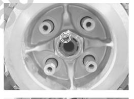
Remove the clutch sleeve hub nut with the special tool. 09920-53730: Clutch sleeve hub holder
