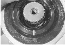
Check the outer race play and smooth rotation of the bearing by hand while it is on the pinion gear shaft.
