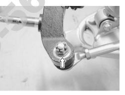
Disconnect the tie rod end with a commercially available ball bearing joint remover ④.
