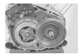
Install the one-way clutch onto the clutch wheel with the  $\rightarrow$  mark facing inside.
