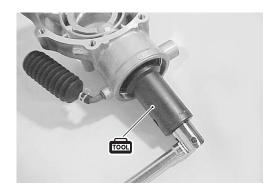
Remove the bearing locknut with the special tool.
