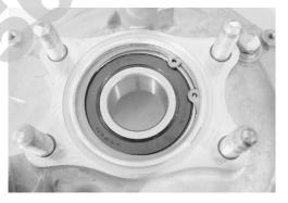
Install new dust seal 2 to the drum cover 3 by using the removed dust seal 1.
