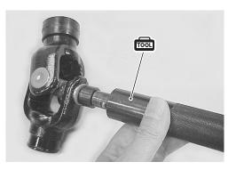
Install new C-rings by tapping with a copper hammer.
