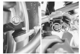
Remove the tie rod ends with a commercially available ball bearing joint remover.
