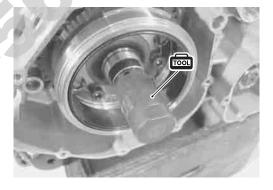
Remove the generator rotor with the special tool. 09930-35010: Rotor remover
