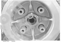
Install the clutch springs and clutch release plate. Tighten the clutch spring bolts diagonally.
