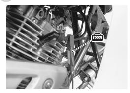
Start the engine and set the engine idle speed between 1 400 and 1 600 r/min by turning the throttle stop screw knob ①.
