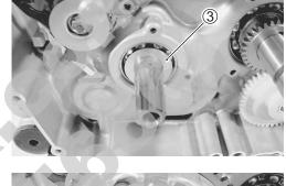
Install the primary driven gear assembly. Install the washer 4.
