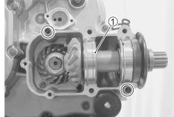
Apply SUZUKI BOND to the mating surface of the secondary bevel gear cover.
