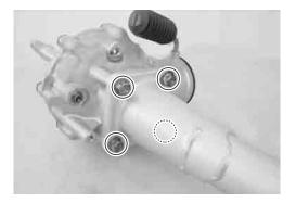
Remove the propeller shaft and spring ③ from the final gear case.
