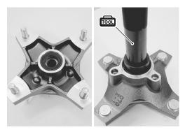
Install the spacer ④ to the front wheel hub.
