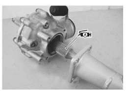
Apply THREAD LOCK SUPER to the axle housing/final gear case bolts, and tighten them to the specified torque.
