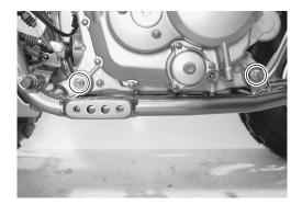
Remove the right front fender bracket (6). Dismount the engine to the right side.
