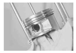
marked side to the top when fitting it to the piston.
