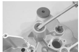
OIL SEAL REMOVAL AND INSTALLATION
