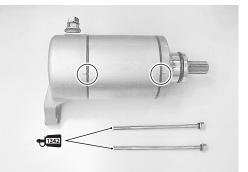
Apply SUZUKI SUPER GREASE to the O-ring.
