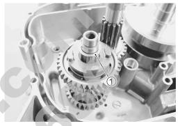
Install the reverse driven gear and washer ②.
