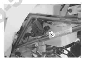
First check the insulation between (A) and (B) terminals with the tester. Then apply 12 V to terminals as shown and check the continuity between (A) and (B). If there is no continuity, replace the neutral relay with a new one.
