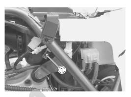
Measure the voltage between the terminals using the multi circuit tester as indicated in the table below.
