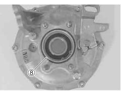
Install the brake panel to the rear axle housing. Install the panel cover (9).
