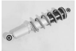
Inspect the rubber bushing for wear or damage.
