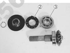
Using a chisel, unlock the nut. Fit the universal joint onto the driven bevel gear shaft. Remove the driven bevel gear shaft by holding the universal joint with a vise.
