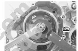
Install the special tool to the crankshaft end. 09930-31921: Rotor remover attachment
