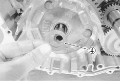
Install the clutch sleeve hub assembly into the primary driven gear assembly.
