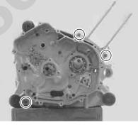
Separate the crankcase with the special tool.
