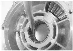
Remove the bearing with the special tool.
