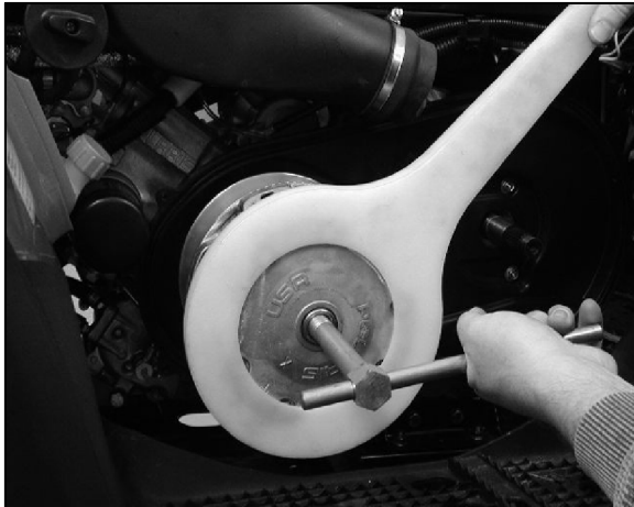
Drive Clutch Puller (PN 2870506) Clutch Holding Wrench (PN 9314177)
