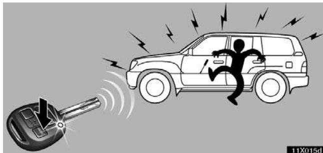
When you push the "PANIC" button for about 1 second, an alarm sounds to deter any person trying to break into or damage your vehicle.
