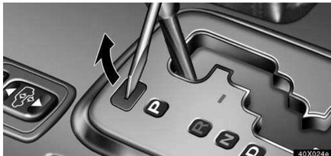
If you cannot shift the selector lever, use the shift lock override button as follows:
