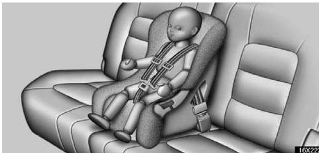
A convertible seat must be used in forward-facing and rear-facing positions depending on the age and size of the child. When installing, follow the manufacturer's instructions about the appropriate age and size of the child as well as directions for installing a child restraint system.
