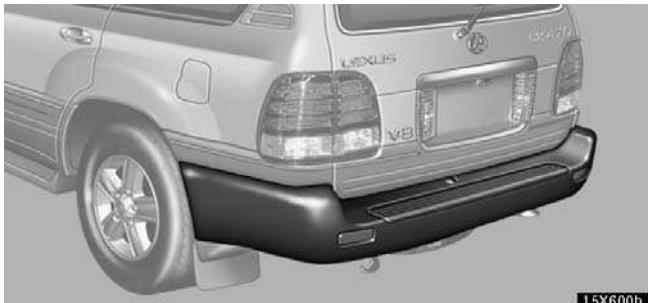
The rear step bumper is for rear end protection and easier step-up loading.
