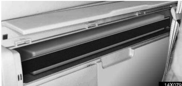
This auxiliary box is equipped with a band to hold the warning reflector.
