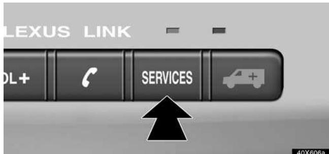
When you push the "SERVICES" button, you will hear "Connecting to Lexus Link". Your location and system ID are automatically transmitted to the advisors that provide services. The services provided will depend on the level of service package selected.
