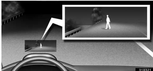
The Lexus night view system can help you see forward when driving at night. If pedestrians or objects are detected within the area reaching the tip of the low beam to high beam, they are displayed along with the layout of the road in the windshield as a monochrome image.
