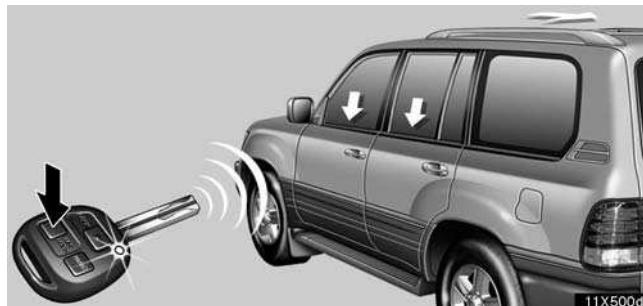
Push the "UNLOCK" button until the windows and moon roof start to move. At this time one beep sounds. When you release the button, the windows and moon roof stop operating.
