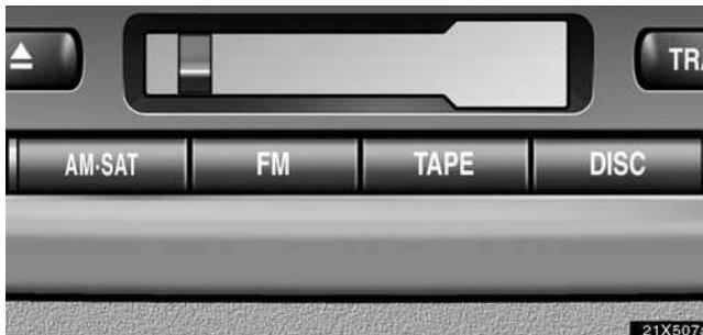
**Push "AM-SAT", "FM", "TAPE" or "DISC" to turn on that mode. The selected mode turns on directly.**
