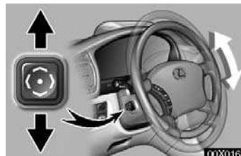
To tilt the steering column up or down to the desired angle, push the control switch in the required direction and release the button when the steering column reaches the desired angle.
