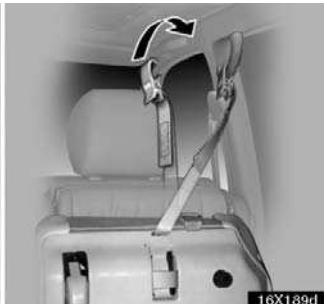
3. Hook the holding strap to the assist grip and secure the seat by pulling its free end.
