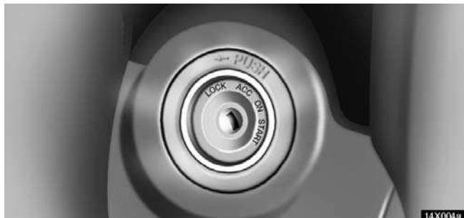
**For easy access to the ignition switch, the ignition switch light comes on when any of the doors are opened.**
