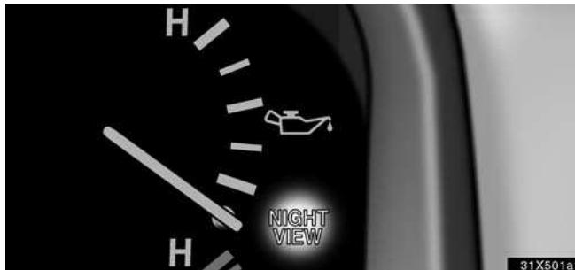
If this warning light comes on, the bulb of the near-infrared floodlight (night view projector) has blown out. Have the bulb replaced at your Lexus dealer.
