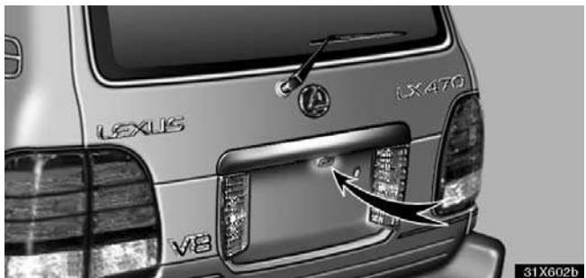
The rear view monitor system camera is located on the back door as shown in the illustration. The camera uses a special lens. The distance of the image that appears on the screen differs from the actual distance.
