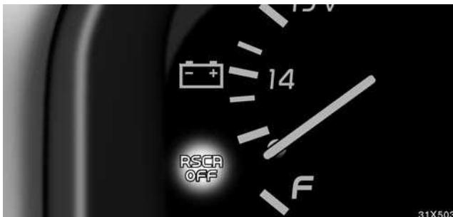
► ***Roll sensing of curtain shield airbags off indicator light***
