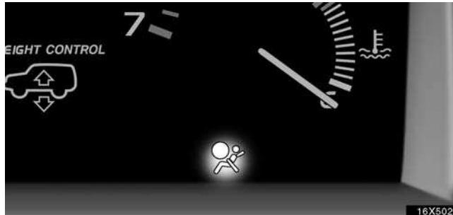
This indicator comes on when the ignition switch is turned to the "ON" position. It goes off after about 6 seconds. This means the SRS side airbags and curtain shield airbags are operating properly.
