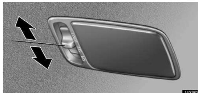
**To turn on the interior light, slide the switch.**
