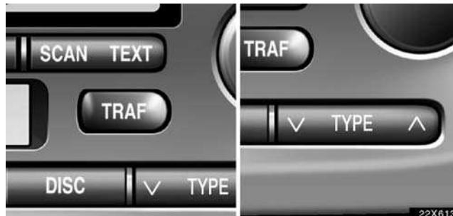
When you push the "TYPE" button, the current program type receiving from RDS station appears on the display.
