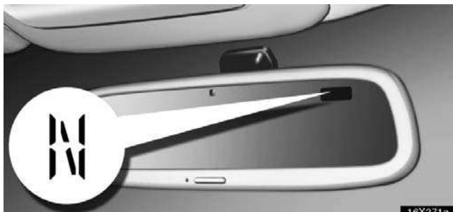
The compass indicates the direction in which the vehicle is heading. The illustration shown above indicates that the vehicle is heading north.
