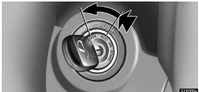
It is not a malfunction if the needles on all meters and gauges move slightly when the key is turned to the "ACC", "ON" or "START" position.
