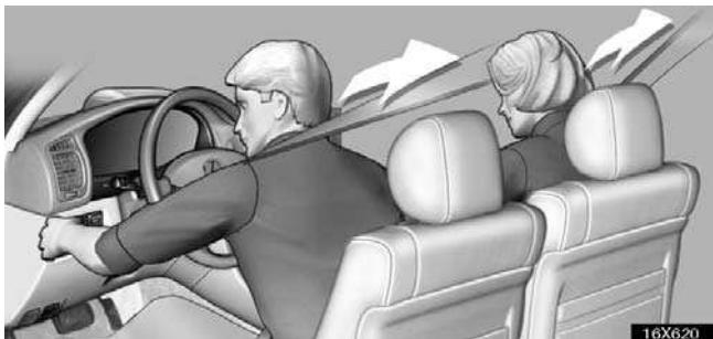
**The driver and front passenger seat belt pretensioners are designed to be activated in response to a severe frontal impact or a vehicle rollover.**
