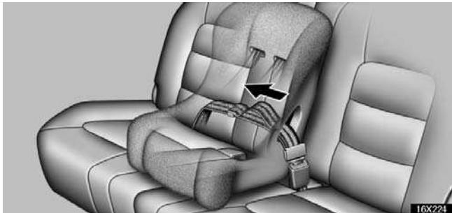
2. While pressing the convertible seat firmly against the seat cushion and seatback, tighten the lap belt by pulling its free end to hold the convertible seat securely.
