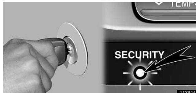
The engine immobilizer system is a theft prevention system. When you insert the key in the ignition switch, the transponder chip in the key's head transmits an electronic code to the vehicle. The engine will start only when the electronic code in the chip corresponds to the registered ID code for the vehicle.
