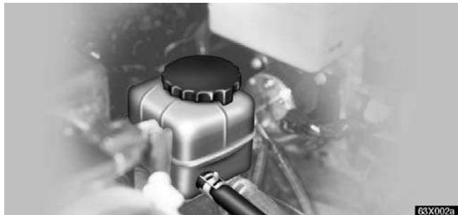
**Check the fluid level on the dipstick. If necessary, add automatic transmission fluid DEXRON® II or III.**
