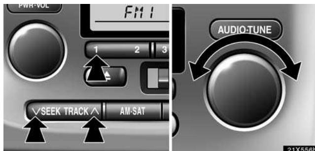
**Preset tuning:** Push the button ( 1–6 ) for the station you want. The button number ( 1–6 ) and station frequency appear on the display.
