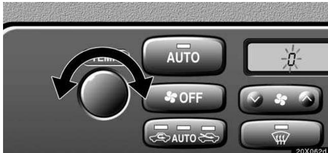
When you turn the "TEMP" knob, the sensitivity changes from "+3" down to "-3". If you do not operate any button for a few seconds or if you push a button other than the air intake control button and temperature control knob, the previous display returns.
