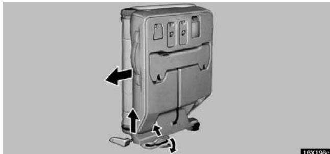
3. Remove the lever cover and pull the lock release lever. Lift up the rear side of the seat and pull the whole seat backward.
