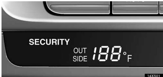
This display shows the outside temperature when the ignition switch is on.
