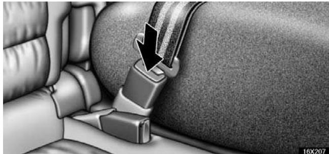
4. To remove the infant seat, press the buckle release button and allow the belt to retract completely. The belt will move freely again and be ready to work for an adult or older child passenger.
