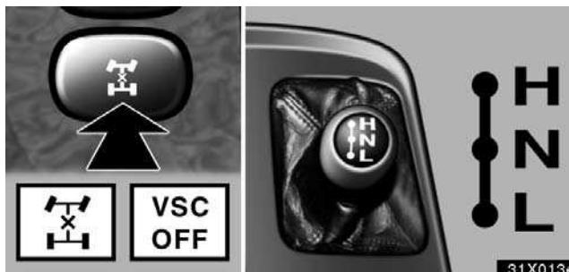
Use the four-wheel drive control lever and center differential lock button to select the following transfer and center differential modes.
