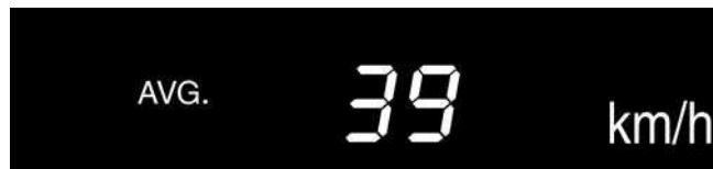
The average vehicle speed is calculated and displayed based on the total driving distance and the total driving time with the engine running.
