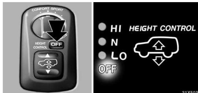
To turn off the active height control suspension with the vehicle stopped, push the height control switch. The height control "OFF" indicator light comes on and the vehicle height is fixed in the same mode as the height control switch is pushed.
