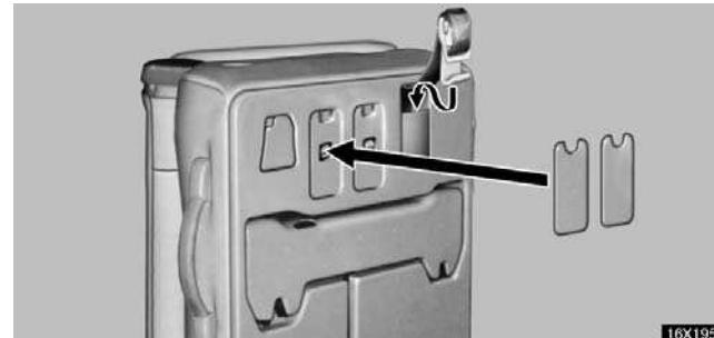
When returning the third seat to its original position, stow the holding strap and the seat hook covers into the holder facing the direction shown in the illustration.
