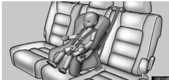
A convertible seat must be used in forward-facing or rear-facing position depending on the age and size of the child. When installing, follow the manufacturer's instructions about the appropriate age and size of the child as well as directions for installing the child restraint system.
