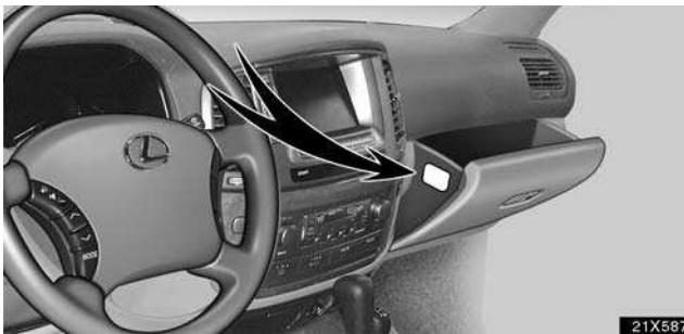
The air conditioning filter information label is placed on the left side of the glove box as shown and indicates that a filter has been installed.
