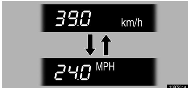
The unit shown on the display can be changed using the following procedure:
