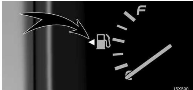
The arrow head next to
