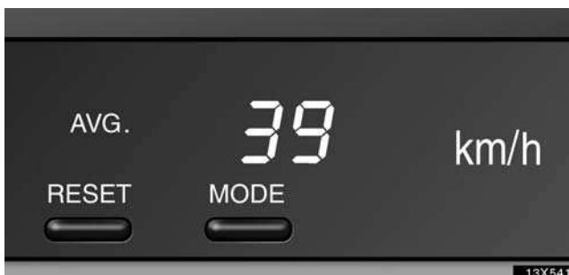
The following information is shown with the ignition switch turned on. Each time you push the "MODE" button, the displayed information is changed.
