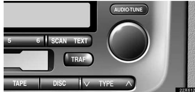
Each time you push the "AUDIO-TUNE" knob, the display changes as in the following. To adjust the tone and balance or turn on or off the automatic sound levelizer, turn the knob.
