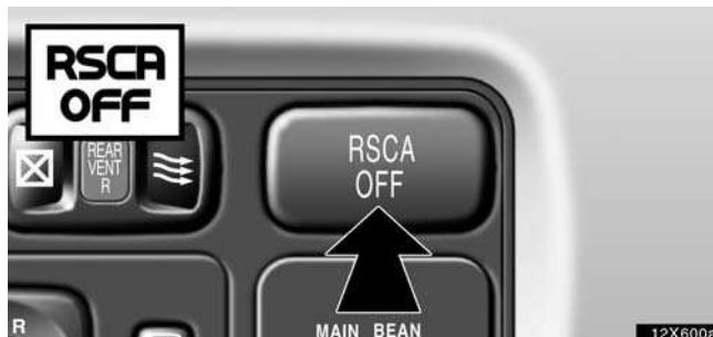
The roll sensing of curtain shield airbags off switch can turn off the curtain shield airbags and front seat belt pretensioners in a vehicle rollover. This switch should only be used in a situation where the inflation is not desired (such as during extreme offroad driving).
