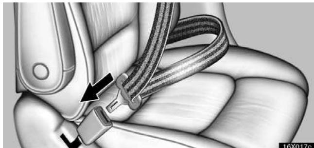
**Adjust the seat as needed and sit up straight and well back in the seat. To fasten your belt, pull it out of the retractor and insert the tab into the buckle.**
