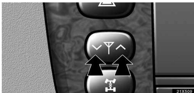
To adjust the height of the antenna manually, push the switch at either side, this may be performed during antenna extension. The maximum extension length is 850 mm (33.5 in.).
