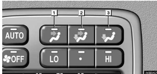
The outlets from which air is delivered can be selected manually by pressing in the appropriate air flow control button. The function of each button is as follows:
