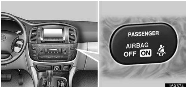
**The front passenger occupant classification indicator light indicates the actuation of the front passenger airbag, side airbag on the front passenger seat and front passenger's seat belt pretensioner.**
