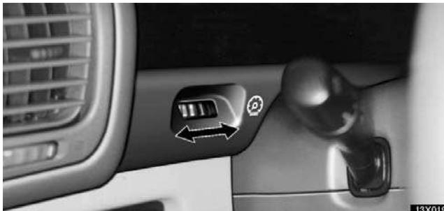
**To adjust the brightness of the instrument panel lights, turn the dial.**
