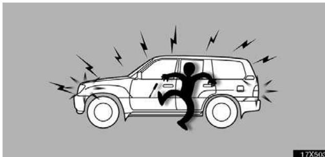
To deter theft of the vehicle, this system is designed to sound an alarm if any of the doors or hood is forcibly unlocked or the battery terminal is disconnected and then reconnected while the vehicle is locked.
