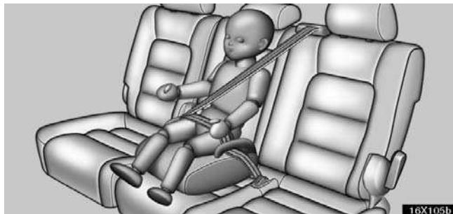
A booster seat must be used in forward-facing position only.
