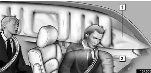
► 1 Curtain shield airbag 2 Side airbag
