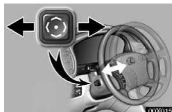
To move the steering column to the desired position, push the control switch away from you or pull it toward you until the steering column reaches the desired position.
