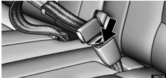
To release the belt, press the buckle release button.
