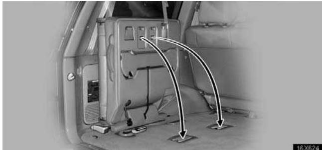
4. Remove the seat hook covers from the back of the seat cushion and install them onto the seat anchor brackets.
