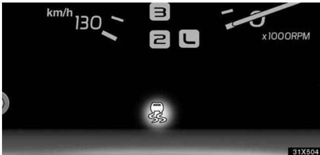
The vehicle stability control system helps provide integrated control of the systems such as anti-lock brakes, traction control, engine control, etc. This system automatically controls the output of the brakes or engine to help prevent the vehicle from skidding under adverse conditions.
