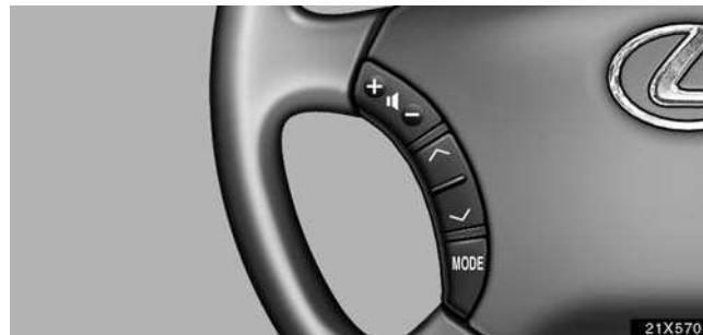
The switches are installed on the left side of the steering wheel.
