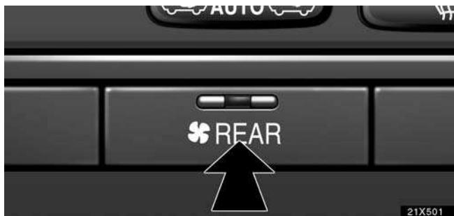
To turn on the rear air conditioning when you sit on the front seat, push this switch. The rear air conditioning operates in the automatic mode. To adjust the air flow and setting temperature, follow the steps in accordance with "Rear air conditioning controls" on page 213.
