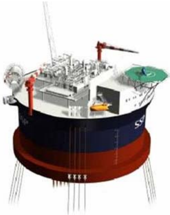
Hull in combination with motion dampening features
