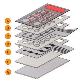
A: Key panel graphics B: 3M<sup>™</sup> Adhesive Transfer Tape C: Top switch circuit D: 3M<sup>™</sup> Membrane Switch Spacer E: Bottom switch circuit F: 3M<sup>™</sup> Adhesive Transfer Tape G: Backer board
