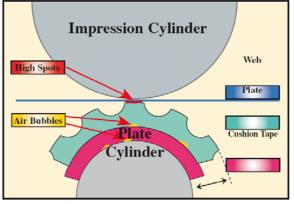
3M<sup>™</sup> E-Series Liner – exclusive liner prevents air entrapment by forming micro-channels in the adhesive.
