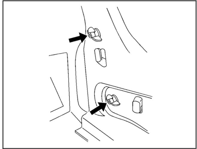
3. Remove the four plastic wing nuts retaining the trunk trim. There are two wing nuts located on the driver's side (shown) and two located on the passenger's side of the vehicle.
