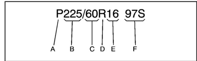
**(A) Passenger (P-Metric) Tire:** The United States version of a metric tire sizing system. The letter P as the first character in the tire size means a passenger vehicle tire engineered to standards set by the U.S. Tire and Rim Association.
