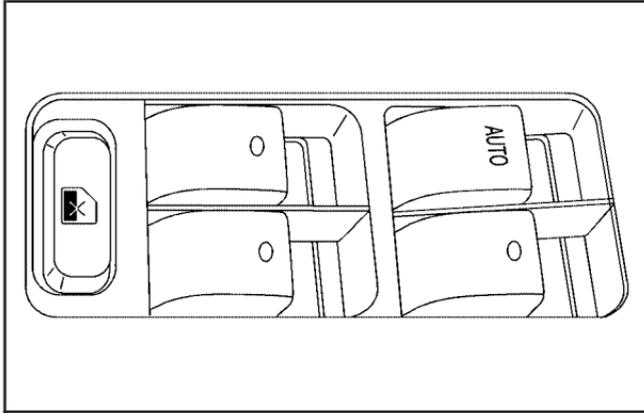
The switches on the driver's door armrest are used to control each of the windows. The power window switches work while the ignition is in RUN, ACCESSORY, or while Retained Accessory Power (RAP) is active. See *Retained Accessory Power (RAP)* on page 110. Each passenger door has its own window switch.
