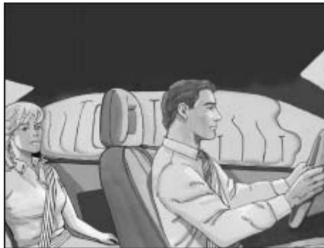
If your vehicle has a roof-mounted side impact airbag for the driver and the person seated directly behind the driver, it is located in the ceiling above the side windows.
