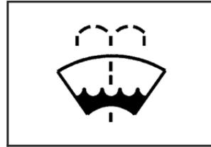
Open the cap with the washer symbol on it. Add washer fluid until the tank is full. See *Engine Compartment Overview on page 350* for reservoir location.
