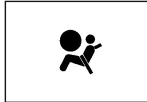
This light will come on when the vehicle is started, and it will flash for a few seconds. Then the light should go out.
