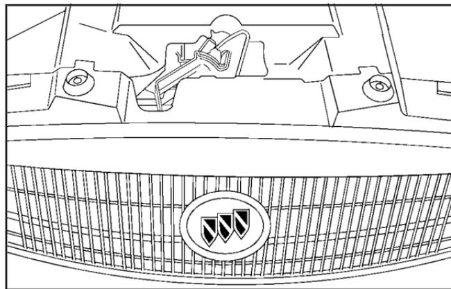
2. Push the secondary hood release lever, located under the center of the hood above the grille, up and to the right to disengage it.
