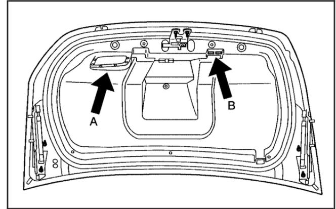
Your vehicle has a trunk lid pull down handle (A) located on the inside of the trunk lid on the driver's side of the vehicle. Use the handle to pull down the trunk lid when closing it.
