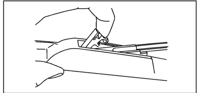
2. While holding the wiper arm, pull the clip up from the blade connecting point, and pull the blade assembly down toward the windshield to remove it from the wiper arm.
