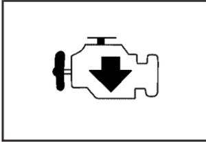
If the reduced engine power light is on, a chime will sound and a noticeable reduction in the vehicle's performance may occur.
