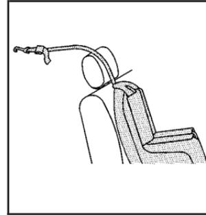
If the position you are using has a fixed headrest and you are using a single tether, route the tether over the head restraint.
