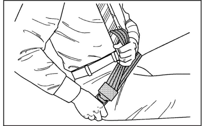
To make the belt shorter, pull its free end as shown until the belt is snug.
