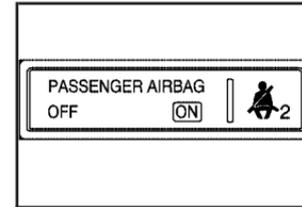
The passenger airbag status indicator will light ON and OFF for several seconds as a system check.
