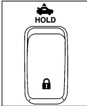
To lock or unlock all doors from inside the vehicle, use the power door lock switch located on either front door armrest.
