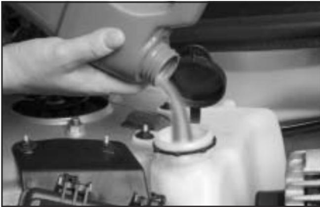
5. Then fill the coolant recovery tank to the cold fill line.
