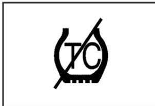
This light, along with the TRACTION CONTROL OFF message, will display on the DIC for three seconds when the ETS is not on.
