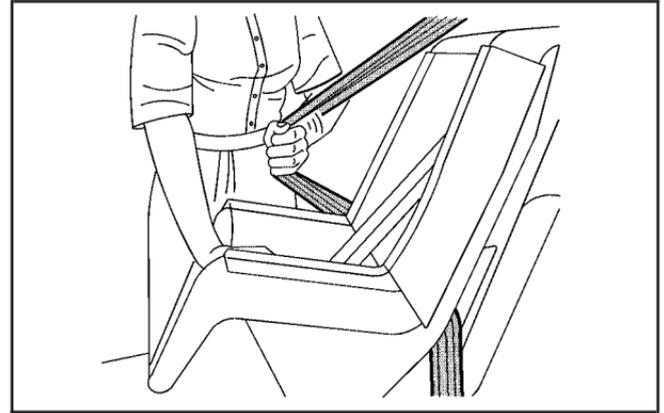
4. Pull the rest of the shoulder belt all the way out of the retractor to set the lock.
