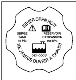
1. You can remove the pressure cap when the cooling system, including the pressure cap and upper radiator hose is no longer hot.
