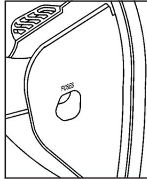
The instrument panel fuse block is located on the passenger's side of the instrument panel. Pull off the cover labeled FUSES to expose the fuse block.
