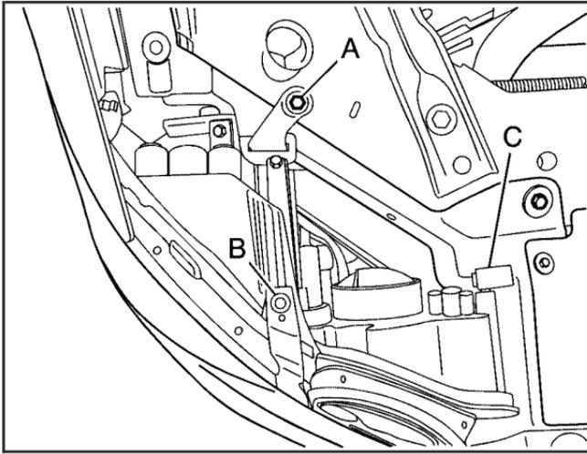
3. Pull up on the plastic retaining clip (C) while pushing rearward on the headlamp. Align the square cut-out on the retaining clip with the notch on the headlamp.
