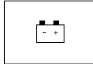
This light comes on briefly when the ignition is turned on, as a check to show that it is working. Then it should go out.
