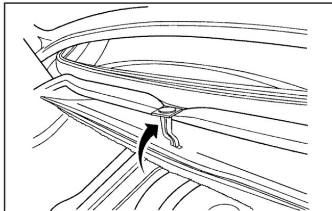
3. Lift the handle on the spare tire cover. The handle may hook on the front edge of the trunk's weatherstrip to hold the cover out of the way.
