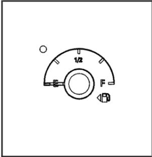
The fuel gage indicates about how much fuel is left in the fuel tank when the ignition is on.
