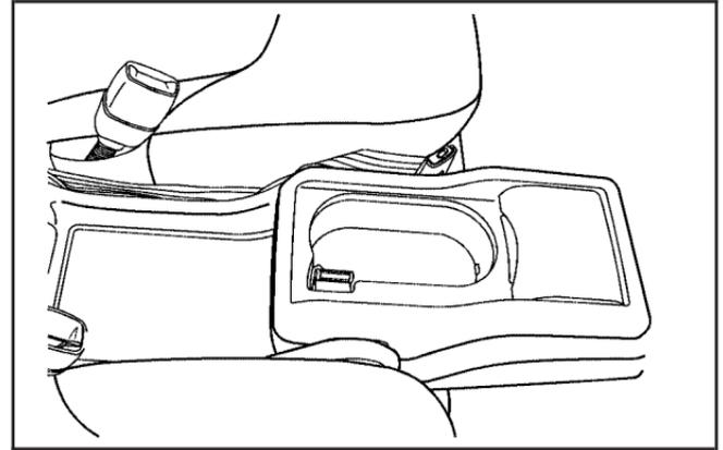
If your vehicle is the six-passenger model, there is a cupholder located underneath the seat. To access, pull the center seat forward. The cupholder has a support that adjusts to two positions to fit either a large cup or two smaller cups.
