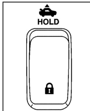
Press and hold the top of the driver's or front passenger's power door lock switch to unlock the trunk.
