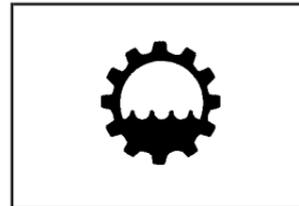
The transaxle fluid dipstick handle has this symbol on it, and is located near the rear of the engine compartment.
