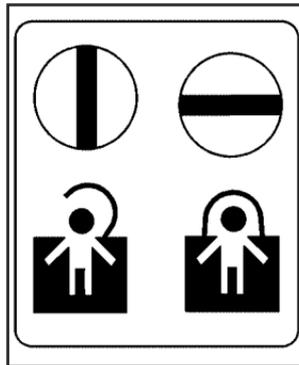
The rear door security locks are located on the inside edge of each rear door. You must open the rear doors to access them.
