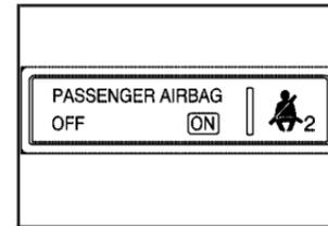
The passenger airbag status indicator will light ON and OFF for several seconds as a system check.
