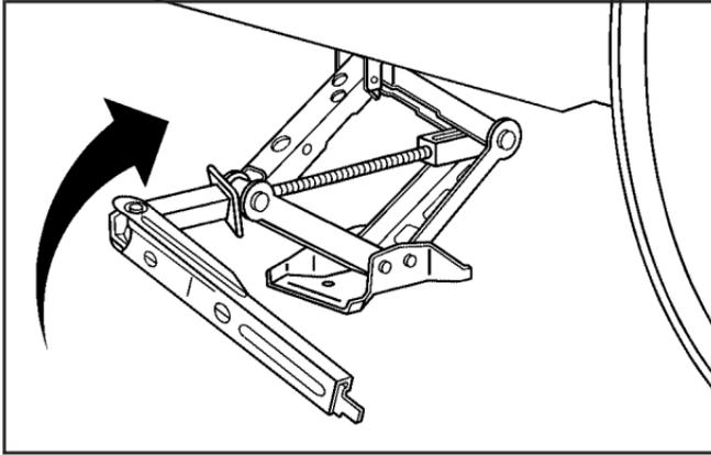
5. Raise the vehicle by turning the jack handle clockwise. Raise the vehicle far enough off the ground for the compact spare tire to fit under the vehicle.
