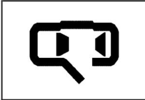
When the ignition is on, this light will stay on until all doors are closed and completely latched.
