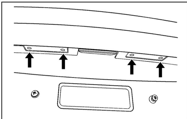
2. Turn and pull the license plate lamp forward through the fascia opening.
