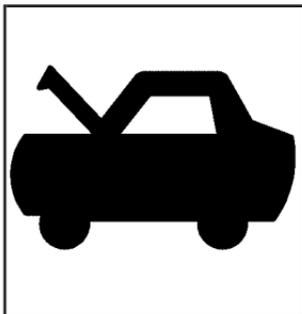
1. Pull the interior hood release handle with this symbol on it. It is located to the left of the steering column below the instrument panel.
