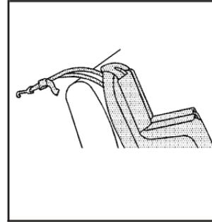
If the position you are using does not have a headrest and you are using a dual tether, route the tether over the seatback.
