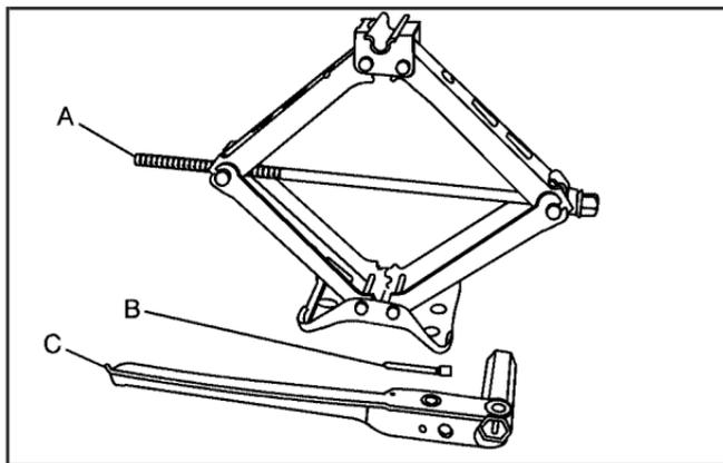
The tools you will need to change a tire include the jack (A), extension and protection guide (B), and wheel wrench (C).
