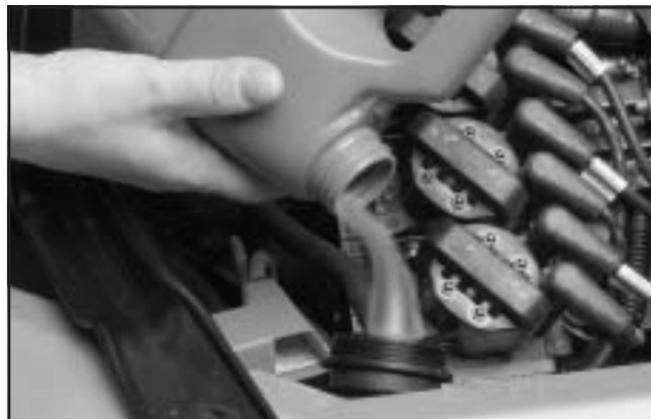
4. Fill the radiator with the proper DEX-COOL<sup>®</sup> coolant mixture, up to the base of the filler neck. See *Engine Coolant* on page 363 for more information about the proper coolant mixture.
