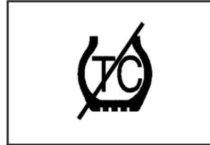
This light, along with the TRACTION CONTROL OFF message, will display on the DIC for three seconds when the TCS is not on.
