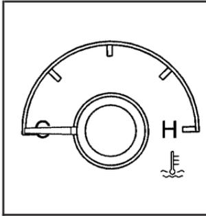
The vehicle has a gage that shows the engine coolant temperature.
