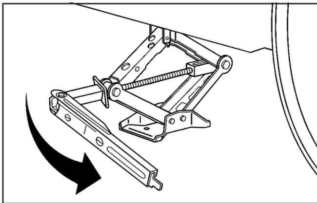
10. Lower the vehicle by turning the jack handle counterclockwise. Lower the jack completely.
