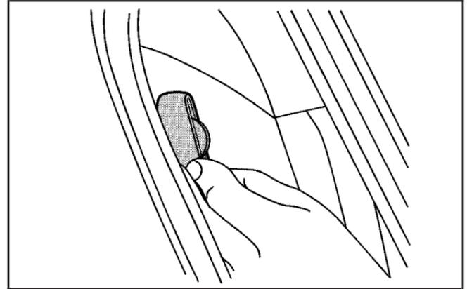
1. Pull the elastic cord out from between the edge of the seatback and the interior body to remove the guide from its storage clip.
