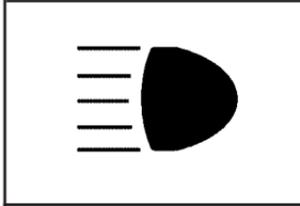
When the high beams are on, a light on the instrument panel cluster also will be on if the ignition is on.
