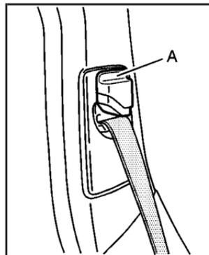
To move it down, press down on the release lever (A) and move the height adjuster to the desired position. You can move the height adjuster up just by pressing up on the shoulder belt guide.
