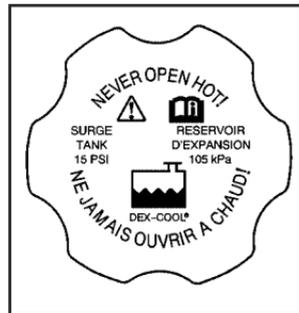
1. You can remove the radiator pressure cap when the cooling system, including the radiator pressure cap and upper radiator hose, is no longer hot.
