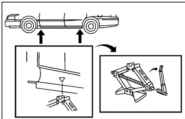
3. Find the jacking location using the diagram above and corresponding triangular-shaped hoisting notches located on the underside of the vehicle's plastic molding.
