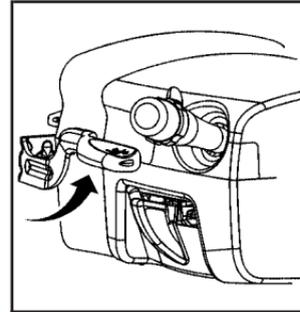
The lever that makes this adjustment is located on the left side of the steering column and behind the tilt lever, if the vehicle has this feature.
