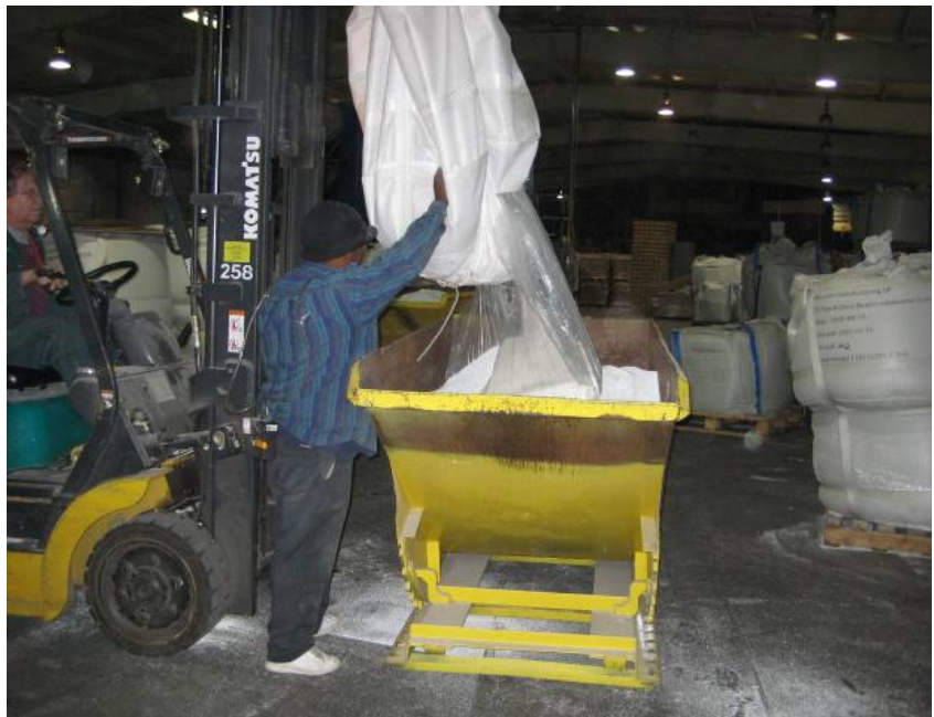
Figure 1. Employee emptying a Super Sack® into a bin
