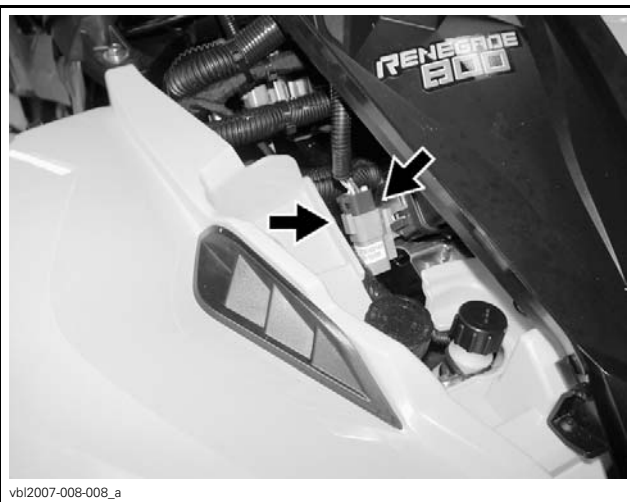
vbi2007-008-008_a RENEGADE SERIES (TYPICAL) Step 1: Remove seat Step 2: Remove central panel
