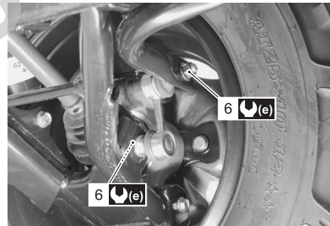
6 (e) Rear stabilizer joint nut 60 N-m (6.0 kgf-m, 43.5 lbf-ft)
