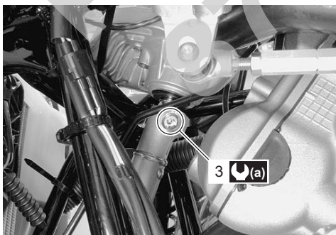
3 (a) Steering shaft bolt 26 N-m (2.6 kgf-m, 19.0 lbf-ft)
