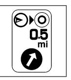
The straight line to distance symbol indicates the straight-line distance to the destination.
