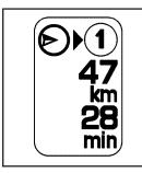
The distance and time to destination symbol indicates the distance and the estimated time remaining to the final destination, depending on the option selected.
