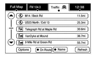
Press the NAV key, then press the NAV key repeatedly until Traffic is selected, or touch the Traffic screen button. A list of traffic conditions may display with the direction and how far away the traffic conditions are from the vehicle's current position.
