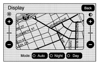
Select this screen button to change the brightness, contrast, and mode of the display.
