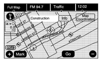
While scrolling the map, traffic condition icons may appear. To receive information about the traffic condition, place the cross hairs over the traffic condition icon. After selecting the INFO (information) screen button, the type of traffic condition, the street name, and a description of the traffic condition displays. See "Scrolling the Map" under *Maps on page 2-4* for more information.
