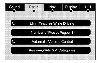
Press the MENU key to enter the configure menu screen, then press it repeatedly until Radio is selected, or select the Radio screen button to make changes for radio information displayed, number of preset pages, XM categories, if equipped, and automatic volume control.
