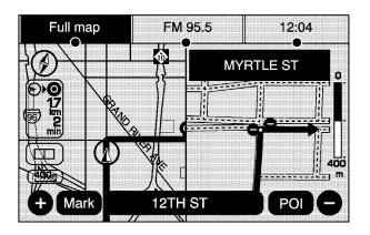
When you are approximately 1/4 mi (400 m) from the next maneuver in city driving, the screen displays the name and a detailed view of the next maneuver. On the freeway, these details appear at 1 mi (1200 m) from the maneuver.
