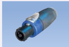
Adapter - NL4FC to 1/4 Inch 2-pole jack, wiring: +1 to TIP and -1 to SLEEVE - pre-wired Part #: NA4LJX
