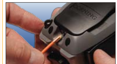
Step 5 : Crimp the Connectors onto the Fiber
