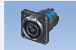
Receptacle Speakon® STX - 4 pole female - solder cups - black/silver.
