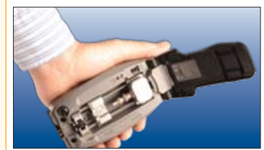
Step 1 : Place the Connector in the Tool
