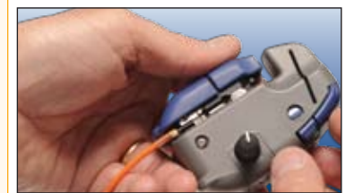
Step 4 : Cut Fiber to Proper Length
