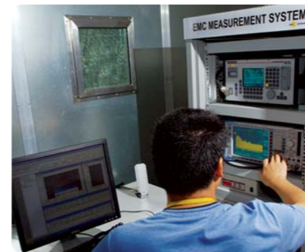
This is the Electromagnetic chamber where we test all products for compliance with standards such as FCC emissions, CE and safety. The facility represents a multi-million dollar investment and includes at least one machine that goes "ping"
