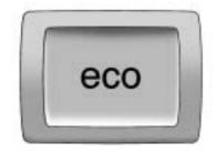
Press the "eco" (economy) button by the shift lever to turn this feature on or off. The "eco" light in the instrument cluster will come on when engaged. See *Fuel Economy Light on page 4-25*. For vehicles with a Driver Information Center (DIC) an "ECO Mode On" message displays. See *Fuel System Messages on page 4-35* for more information.
