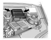
To remove the fuse block cover, squeeze the clips on the cover and lift it straight up.
