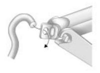
8. Fit the jack handle extension onto the jack by sliding the hook through the end of the jack.
