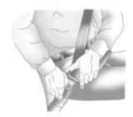
To unlatch the belt, push the button on the buckle. For outboard seating positions, slide the latch plate up the safety belt webbing when the safety belt is not in use. The latch plate should rest on the stitching on the safety belt, near the guide loop.
