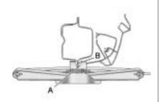
Place the jack notch (A) under the frame rail seam (B).
