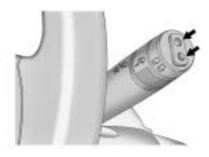
Press the upper or lower portion of the button to control the rear wiper and rear wiper delay. The system turns off when the button is returned to the middle position.
