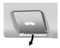
Pull the release handle with the symbol on it. It is below the instrument panel, to the left of the steering wheel.
