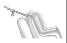
If the position you are using does not have a headrest or head restraint and you are using a single tether, route the tether over the seatback.
