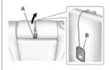
Stow the rear seat center armrest. Attach the retaining strap to the armrest loop (A) and to the center top tether anchor on the seatback (B). Make sure the retaining strap's clips are firmly attached.
