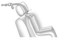
If the position you are using has a fixed headrest or head restraint and you are using a single tether, route the tether over the headrest or head restraint.
