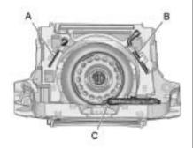
Remove the extension (A), wheel wrench (B) and jack (C).
