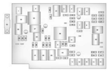
**Engine Compartment Fuse Block**
