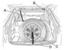
4. Pull the cable (A) through the door striker (D) then the center of the wheel (C).
