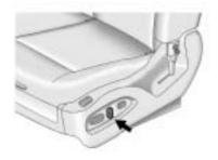
On vehicles with power reclining seatbacks, the switch is located on the outboard side of the seat. See *Power Seat Adjustment on* page 2-4 for more information.
