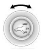
Choose the power liftgate mode by turning the dial on the switch until the indicator lines up with the desired position. The vehicle must be in P (Park).
