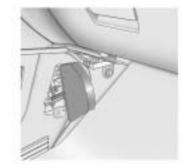
The instrument panel fuse block is located on the passenger side panel of the center console. To access the fuses, open the fuse panel door from the passenger side by pulling it out.
