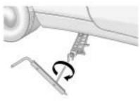
11. Raise the vehicle by turning the jack handle clockwise. Raise the vehicle far enough off the ground so there is enough room for the road tire to clear the ground.
