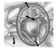
The adjustment lever is located on the left side of the steering column.
