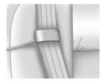
The belt should not be twisted and it should lie flat. The elastic cord must be under the belt and the guide on top.
