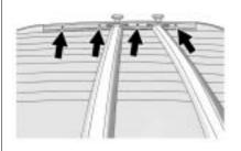
The roof rack crossrails can be locked in four positions along the roof rack side rails.
