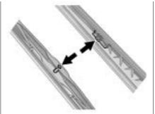
Place the wiper blade into the wiper arm aligning the blade attachment rivet with the arm attachment.
