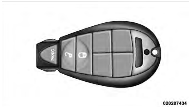
Key Fob With Three-Button RKE Transmitter
