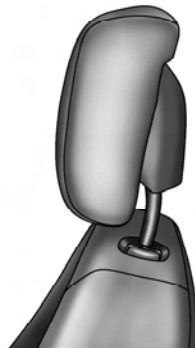
Active Head Restraint (Normal Position)
