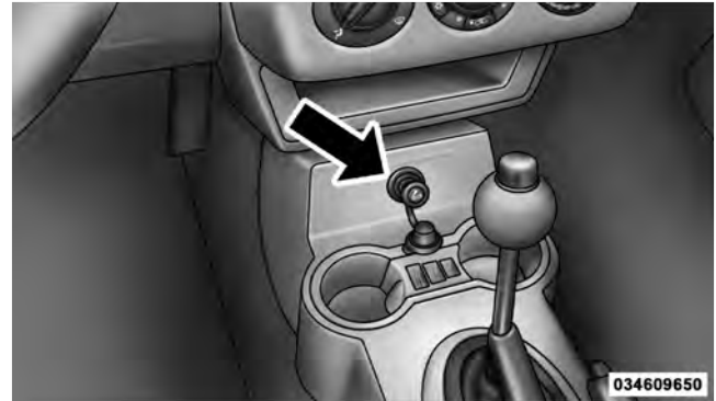
Front Power Outlet
