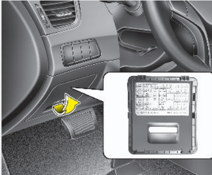
Inner panel fuse panel
