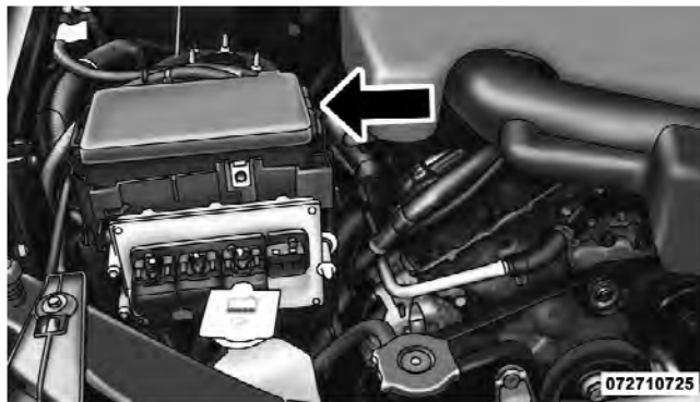
Totally Integrated Power Module
