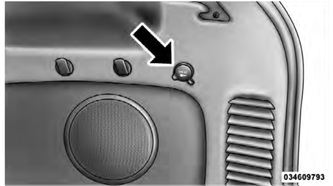
Rear Power Outlet
