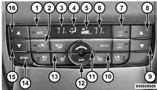
Automatic Temperature Control (ATC) Panel
