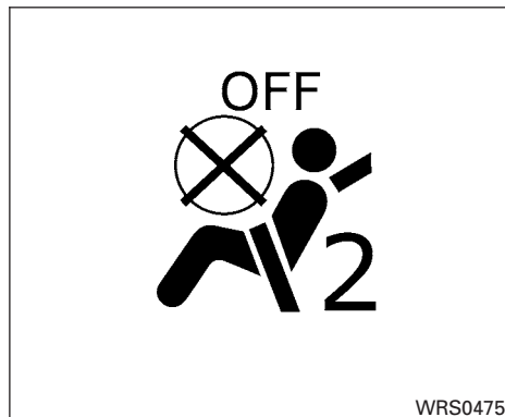
Front passenger air bag and status light
