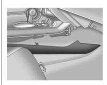
Pull the passenger side console trim away from the front half of the console to expose the shift lever mechanism.
