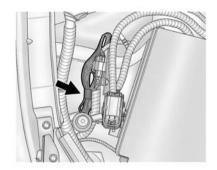
The electrical cord is located on the passenger side of the engine compartment, next to the engine compartment fuse block for V6 models
