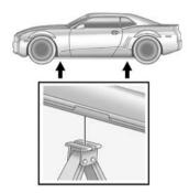
4. Position the jack lift head at the jack location nearest the flat tire. The location is indicated by a mark on the bottom edge of the vehicle. The jack must not be used in any other position.
