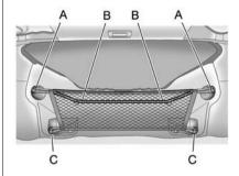
The upper (A) and lower (C) hooks on each side of the trunk opening are provided to attach the net.
