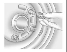
Remove all of the wheel nuts and place them in a dry, clean place to avoid getting dirt in the threads.
