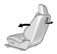
To access the rear seats, pull up on the latch on the rear of the driver or front passenger seatback. Fold the seatback forward.
