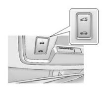
**Open/Close:** Press and hold the rear or front of the switch to open or close the sunroof.
