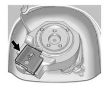
The tire sealant and compressor kit is located in a foam container in the trunk.
