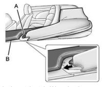
4. Insert the tab (A) under the trim (B) on both sides.
