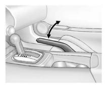
To apply the parking brake, pull up on the parking brake handle. It is not necessary to push in on the release button while applying the parking brake. If the ignition is in the ON/RUN position, the brake system warning light will come on. See Brake System Warning Light on page 5-18.
