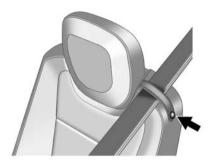
If the seat has a safety belt guide, and the safety belt is not routed through the guide, snap the guide around the belt webbing. Be sure the belt is not twisted.
