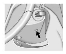
Vehicles with an automatic transmission are equipped with an electronic key lock release system. The key lock release is designed to prevent ignition key removal unless the shift lever is in P (Park).
