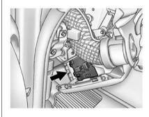
The instrument panel fuse block is located on the end of the instrument panel, on the driver side of the vehicle. To access the fuses, open the fuse panel door by pulling out.
