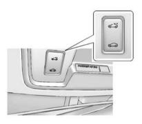
**Open/Close:** Press and hold the rear or front of the switch to open or close the suproof
