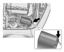
To remove the hinged fuse block cover, press the clip at the front of the cover, and swing it up.
