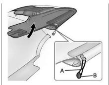
Fold the sides of the tonneau cover over. Attach the cord (A) at the front edge of the tonneau cover to the post (B) on the back seat rear panel on both sides.
