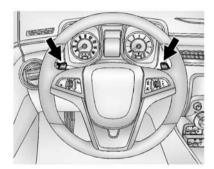
Tap Shift allows the driver to manually control the automatic transmission. To use Tap Shift, the shift lever must be in M (Manual Mode). Vehicles with this feature have indicators on the steering wheel. The controls are on the back of the steering wheel. Tap the left control to downshift, and the right
