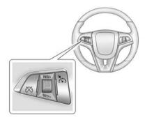
The cruise control buttons are located on the outboard side of the steering wheel.
