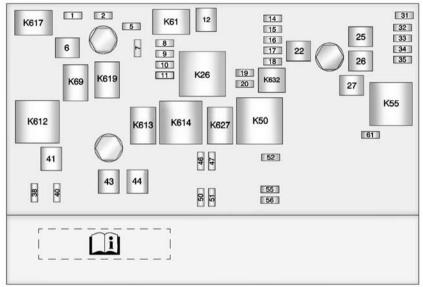
**Engine Compartment Fuse Block**
