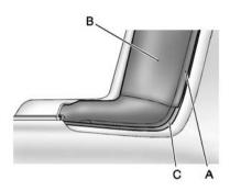
6. Push the edge (A) of the center of the tonneau cover (B) under the vehicle trim (C).
