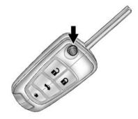
Press the key release button to extend the key blade. The key can be used for the ignition and all locks.
