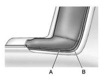
5. Push the outside rim (A) of the tonneau cover under the vehicle trim (B) on both sides.
