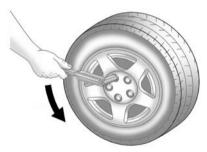
Use the fully extended wheel wrench to loosen all the wheel nuts one-half turn counterclockwise. Do not remove them yet. Notice: Make sure that the jack lift head is in the correct position or you may damage your vehicle. The repairs would not be covered by your warranty.
