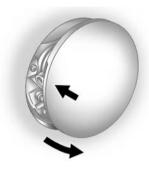
The fuel cap is located behind a hinged fuel door on the passenger side of the vehicle. To open the fuel door, push the rearward center edge in and release and it will open.
