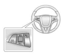
The cruise control buttons are on the outboard side of the steering wheel.
