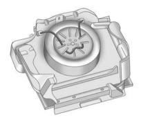
6. Route the strap provided, as shown, to secure the flat tire.
