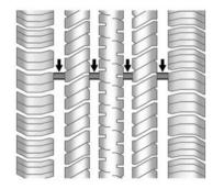
Treadwear indicators are one way to tell when it is time for new tires. Treadwear indicators appear when the tires have only 1.6 mm (1/16 in) or less of tread remaining. See *Tire Inspection on page 10-60* and *Tire Rotation on page 10-60* for more information.
