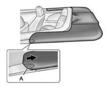
Grip the tonneau cover at the notch (A) and pull back to release the tab on both sides.
