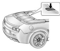
Remove the trim cover to access the hydraulic pressure release bolt.
