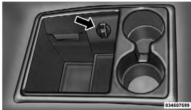
Power Outlet — Floor Storage Bin
