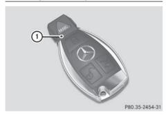
If battery check lamp ① does not light up briefly during the test, the battery is discharged.
