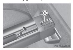
► Make sure that red lock status indicator ④ is no longer visible. The combined cargo cover and net will otherwise not be locked in place.
