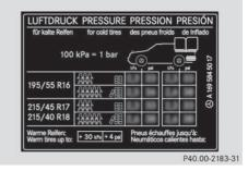
Example: tire pressure table with tire dimensions Some tire pressure tables show only the rim diameters instead of the full tire size, e.g. **R18**. The rim diameter is part of the tire size and can be found on the tire sidewall (> page 368).
