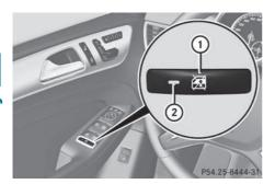
► To activate/deactivate: press button ①. If indicator lamp ② is lit, operation of the rear side windows is deactivated. Operation is only possible using the switches in the driver's door. If indicator lamp ② is off, operation is possible using the switches in the rear compartment.
