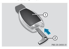
► Press mechanical key ② into the opening in the SmartKey in the direction of the
