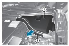
▶ Remove seal (2) in the area around cover (1) in the direction of the arrow.
