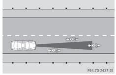
DISTRONIC PLUS has not yet detected the vehicle in front on the edge of the road,
