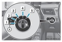
Illustration: light switch with the A symbol for the automatic headlamp mode/daytime running lamps
