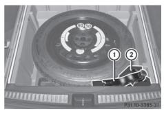
Ball coupling and ball coupling stowage well (example)
