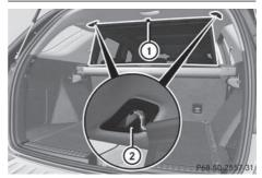
▶ Pull the cargo net up by tab ① and hook it into eyelets ② using both hands.
