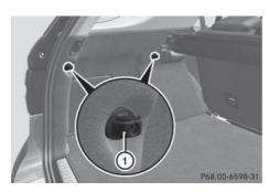
There are two securing hooks ① on each side of the cargo compartment.
