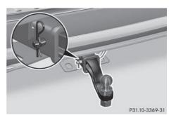
Correctly installed and secured ball coupling ▶ Check the ball coupling, bolt and spring cotter for correct installation.
