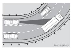
The ability of DISTRONIC PLUS to detect vehicles when cornering is limited. Your vehicle may brake unexpectedly or late.
