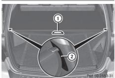
➤ To extend: pull the cargo compartment cover back by grab handle ① and clip it into retainers ② on the left and right.
