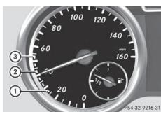
DISTRONIC PLUS displays in the speedometer When DISTRONIC PLUS is activated, one or two segments (2) in the set speed range light up.
