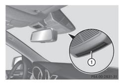
► Fold down the camera cover by recess (1).
