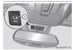
Press and hold Roadside Assistance button (1) for more than two seconds. This initiates a call to the Mercedes-Benz Customer Assistance Center. The indicator lamp in Roadside Assistance button (1) flashes while the call is active. The Connecting Call message appears in the multifunction display. The audio output is muted.
