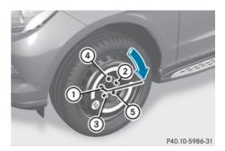
▶ Tighten the wheel bolts evenly in a crosswise pattern in the sequence indicated (1) to (5)). The tightening torque must be 110 lb-ft (150 Nm).
