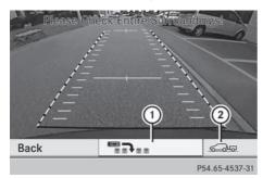
▶ To change the function mode: using the COMAND controller, select symbol (1) for the "Reverse parking" function or symbol (2) for the "Coupling up a trailer" function. See the separate COMAND operating instructions.
