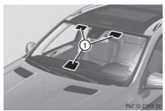
In order to operate radio-controlled equipment, e.g. toll recording systems, areas ① on the windshield are permeable to radio waves. In these areas, you can install radio-controlled systems.
