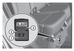
115 V socket (1) provides an alternating voltage of 115 V, so that small electronic devices can be connected. These devices, such as games consoles, chargers and laptops, together should not consume more than a maximum of 150 W.
