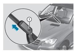
► Firmly press release knob (1) and pull the wiper blade upwards from the wiper arm in the direction of the arrow.
