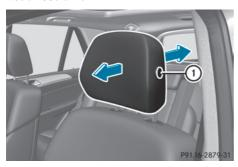
With this function you can adjust the distance between the head restraint and the back of the seat occupant's head.
