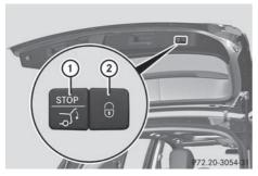
Closing button and locking button (example: vehicle with the EASY-PACK tailgate and KEYLESS-GO)
