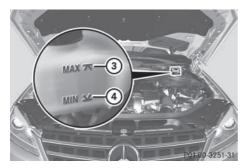
The brake fluid level is correct if it is between MIN marking (4) and MAX marking (3) on the brake fluid reservoir.
