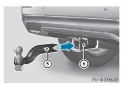
Hole in the ball coupling and ball coupling recess
