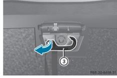
► Fold out hook ③ on the underside of the trunk floor in the direction of the arrow.
