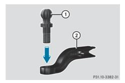
▶ Insert ball coupling (1) through the hole in ball coupling carrier (2) as far as it will go.
