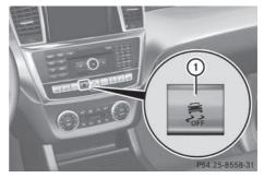
▶ To deactivate: press button (1). The ESP® OFF warning lamp in the instrument cluster lights up.
