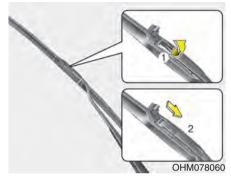
Open the cover of the blade. Press the clip behind the wiper arm and remove the blade assembly downward.
