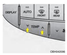
2. Press the TEMP button to set the desired temperature.
