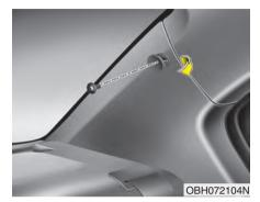
3. Remove the cap, then loosen the mounting screw.
