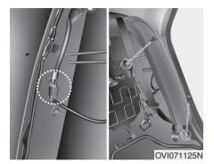
6. Loosen the mounting bolts, then disconnect the connector.
