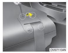
5. Push the hook, remove the rear seat belt cover.
