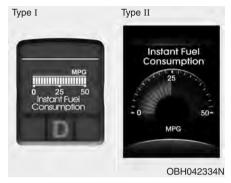
Instant fuel consumption (MPG or I/100km) This mode calculates the instant fuel consumption every 0.2 second from the driving distance and quantity of fuel consumed.
