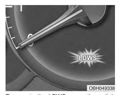
To operate the LDWS, press the switch with the ignition in the ON position. The indicator illuminates on the cluster. To cancel the LDWS, press the switch again.
