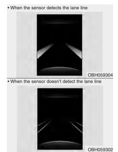
If your vehicle leaves the lane when the LDWS is operating and vehicle speed exceeds 43 mph (70 km/h), the warning operates as follows:
