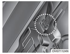
5. Push the hook, disconnect the main connector.
