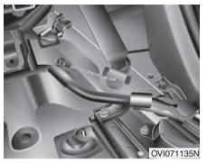
6. Remove the rear seat belt lower anchor.
