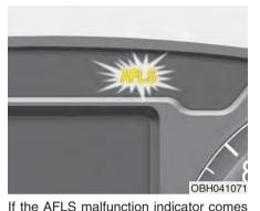
on, the AFLS maintration indicator comes on, the AFLS is not working properly. Drive to the nearest safe location and restart the engine. If the indicator continuously remains on, take your vehicle to an authorized HYUNDAI dealer and have the system checked.
