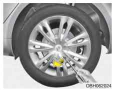
Insert the jack handle into the groove of the wheel cap and pry gently to remove the wheel cap (If equipped).
