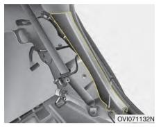
2. Loosen the mounting screw, then remove the rear wheel house trim.
