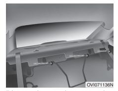
7. Loosen the mounting screws, then remove the package tray trim.
