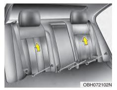
3. Loosen the mounting bolts, then remove the rear seat back.
