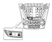
There is a power door lock switch on the instrument panel.
