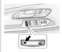
(Window Lockout): This feature prevents the rear passenger windows from operating, except from the driver position.
