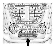
The DIC buttons are located below the climate control system.
