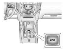
Press the "eco" (economy) button by the shift lever to turn this feature on or off. The "eco" light in the instrument cluster will come on when engaged. See Fuel Economy Light on page 5-19. A Driver Information Center (DIC) message "ECO MODE ON" is also displayed. See Fuel System Messages on page 5-27 for more information.
