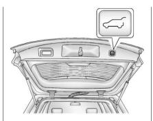
Press and release on the liftgate adjacent to the latch to close the liftgate.
