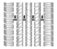
Treadwear indicators are one way to tell when it is time for new tires. Treadwear indicators appear when the tires have only 1.6 mm (1/16 in) or less of tread remaining. See *Tire Inspection on page 10-50* and *Tire Rotation on page 10-51*.
