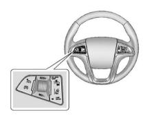
To turn LDW on and off, press the LANE DEPART button, located on the steering wheel.
