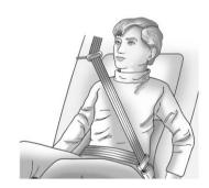
4. Buckle, position, and release the safety belt as described previously in this section. Make sure the shoulder portion of the belt is on the shoulder and not falling off of it. The belt should be close to, but not contacting, the neck To remove and store the comfort guide, squeeze the belt edges together so that the safety belt can be removed from the guide. Slide the guide back into its storage pocket located on the side of the seatback.
