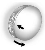
The tethered fuel cap is behind the fuel door on the vehicle's passenger side. To open the fuel door, push the rearward center edge in and release. When applied pressure is removed, the fuel door will spring partially open.
