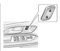
There are power door lock switches on the front door panels.
