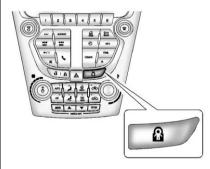
The rear door safety locks switch is on the instrument panel.
