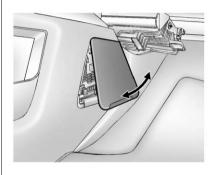
The instrument panel fuse block is located on the passenger side panel of the center console. To access the fuses, open the fuse panel door from the passenger side by pulling it out.
