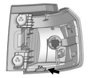
Verify that the taillamp assembly tab, located at the bottom of the taillamp assembly, is aligned to the fascia bracket before securing with screws.
