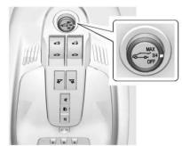
On vehicles with a power liftgate, the vehicle must be in P (Park) to use the power feature. The taillamps flash when the power liftgate moves.
