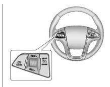
**ON/OFF**  $\ \ \ \ \ \ \ \ \ \ \ \$  Press to turn the cruise control system on and off.
