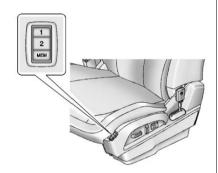
If available, the "1" and "2" buttons on the outboard side of the driver seat are used to manually save and recall the driver seat and outside mirror positions. These manually stored positions are referred to as Button Memory positions.
