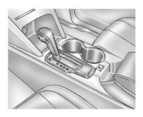
The automatic transmission shift lever is located on the console between the seats.
