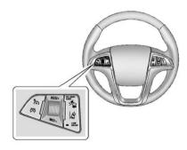
The Collision Alert control is on the steering wheel. Press COLLISION ALERT to set the alert timing to far, medium, near or off. The first button
