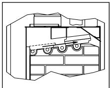
Figure 2b - Top Baffle Removal
