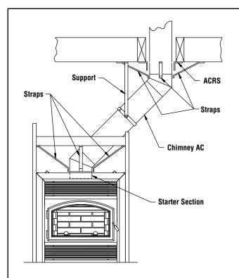
NOTE: This illustration is not to scale. It represents how the chimney must be supported. A 30 degree offset only is allowed in the USA and a 45 degree maximum offset is allowed in Canada.
