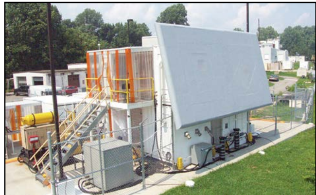
The Advanced Multifunction RF Concept (AMRFC) test bed is a proof-of-principle demonstration system capable of simultaneously transmitting and receiving multiple beams from common transmit and receive array antennas for radar, electronic warfare, and communications. This testbed will be expanded to support the FlexDAR program.
