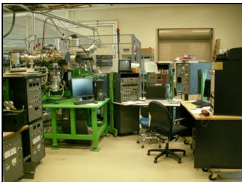
The Secondary Ion Mass Spectrometer/Single-Stage Accelerator Mass Spectrometer performs spatially resolved composition analysis using secondary ion mass spectrometer (SIMS) to sputter atoms, and single stage accelerator mass spectrometer (SSAMS) to reduce background interferences from commonly present molecular ions. Provides high-sensitivity and high-precision measurements.
