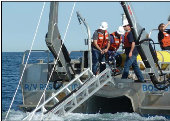
NRL's "Reliant" unmanned undersea vehicle with towed acoustic array being deployed during a long range active acoustics experiment.
