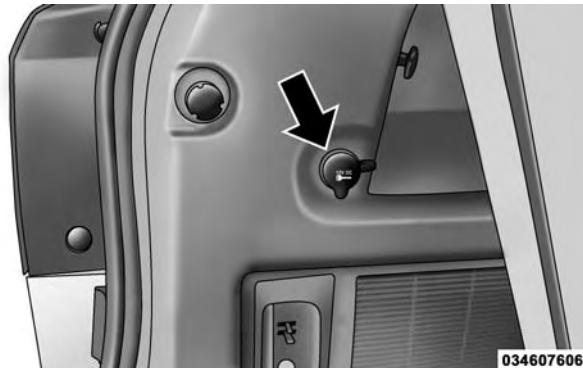
Rear Cargo Area Power Outlet
