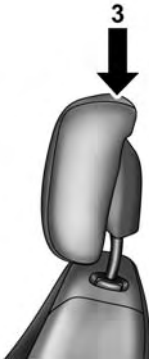
3 — Final Downward Movement To Engage Locking Mechanism
