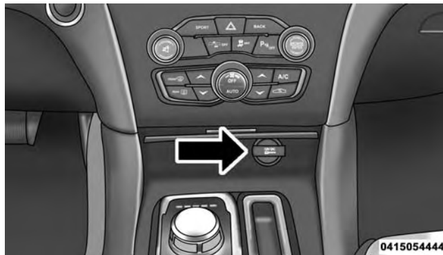
Front Power Outlet
