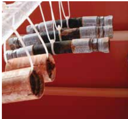
Salt spray test
