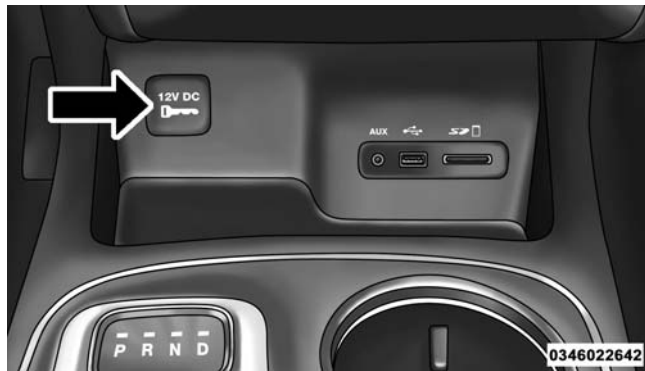
Front Power Outlet
