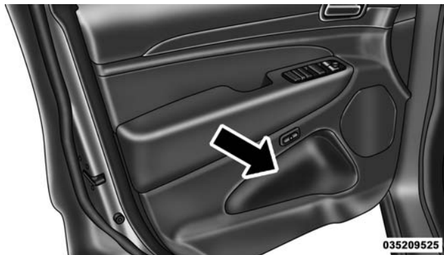
Door Panel Storage
