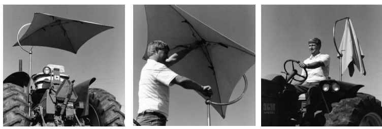
Provides maximum space for standing operator. Tilts to any angle. Folds to one side when not in use.
