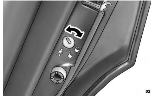
Child-Protection Door Lock Function
