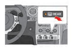
window, be careful not to scratch or damage the rear window defroster.
