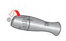
If the ignition switch is pushed to the OFF position and one of the doors is opened, the headlights remain on for 45 seconds.
