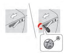
With the outside door handle lifted up, use the mechanical key and turn the key cylinder cap (A) counterclockwise to remove.
