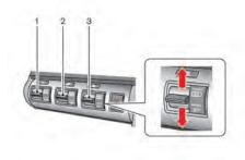
The control of the dual clutch transmission. Bilstein DampTronic® electronically controlled shock absorbers and Vehicle Dynamic Control (VDC) can be changed to the desired modes by operating the setup switches. Select the desired mode best suited to the driving conditions.
