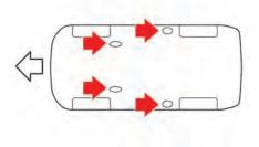
Do not use the tie down hooks for towing or vehicle recovery.
