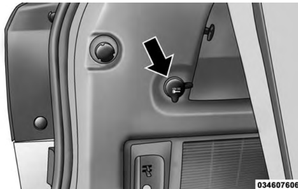
Rear Cargo Area Power Outlet
