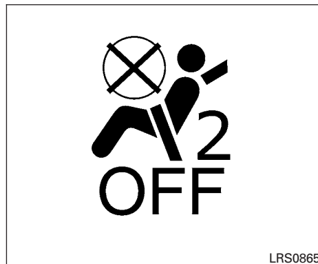
Front passenger air bag and status light
