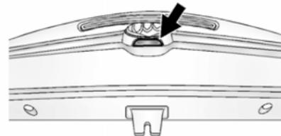
Press the touch pad under the vehicle emblem after unlocking all doors.
