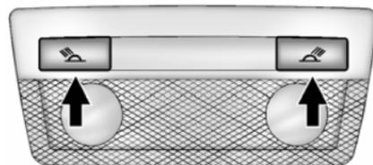
The rear reading lamps are in the headliner.
