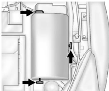
To remove the fuse block cover, press the three retaining clips on the cover and lift it straight up.
