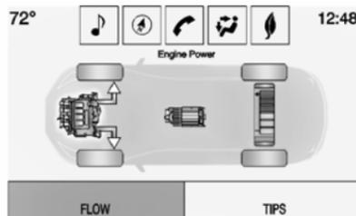
**Engine Power** – Engine is active with energy flowing to the wheels.
