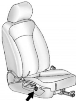
Press and hold the top or bottom of the switch to raise or lower the seat. Release the switch when the desired height is reached.
