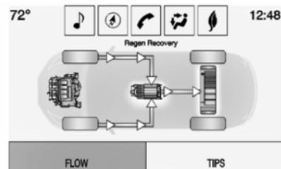
**Regen Recovery** – Power from the wheels returns to the battery during regenerative braking or coasting.
