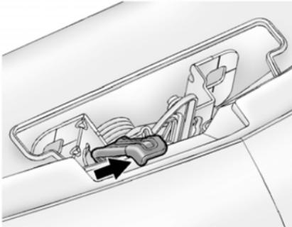
2. Go to the front of the vehicle to find the secondary hood release handle. The handle is under the front edge of the hood near the center. Push the handle to the right and at the same time raise the hood.
