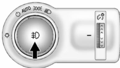
To turn on the fog lamps, if equipped, the ignition and the headlamps or parking lamps must be on.
