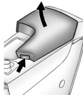
Press the button to access the storage under the armrest. There are two USB ports, an SD card reader, and a power outlet inside. If equipped, there is an auxiliary input jack. See the infotainment manual.
