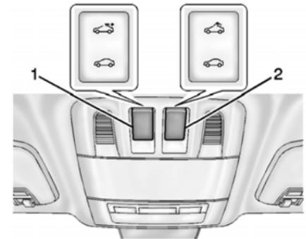
For vehicles with a sunroof, the sunroof only operates when the ignition is in ON/RUN or ACC/ACCESSORY or in Retained Accessory Power (RAP). See *Retained Accessory Power (RAP)* on page 9-23.
