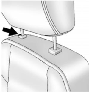
Pull the head restraint up to raise it. To lower the head restraint, press the release button, located on the head restraint post on the top of the seatback, while you push the head restraint down.
