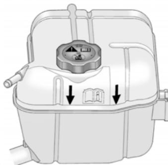
3. Fill the coolant surge tank with the proper DEX-COOL coolant mixture to the indicated level mark.
