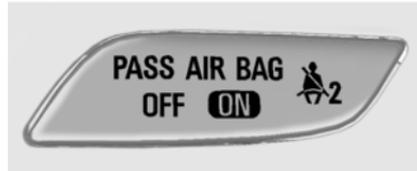
When the vehicle is started, the passenger airbag status indicator will light ON and OFF for several seconds as a system check. Then, after several more seconds, the status indicator will light either ON or OFF to let you know the status of the front outboard passenger frontal airbag.
