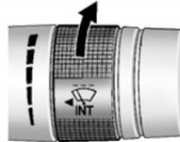
**INT (Intermittent Wipes):** Move the lever up to INT for intermittent wipes, then turn the
