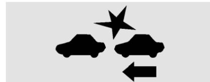
If ACC is engaged, driver action may be required when ACC cannot apply sufficient braking because of approaching a vehicle too rapidly.
