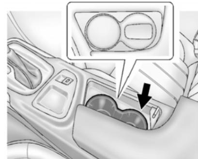
1. Place the recognized transmitter(s) in the cupholder. The cupholder liner will need to be pulled out to access the transmitter pocket.
