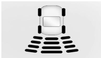
The instrument cluster may have a parking assist display with bars that show “distance to object” and object location information for RPA, and on some vehicles, for the FPA system. As the object gets closer, more bars light up, and the bars change color from yellow to amber to red.
