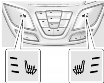
If equipped, the buttons are part of the climate control system on the center stack. To operate, the ignition and the climate control system must be on. If the climate control system is off, press the
