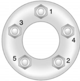
17. Tighten the wheel nuts firmly in a crisscross sequence, as shown.
