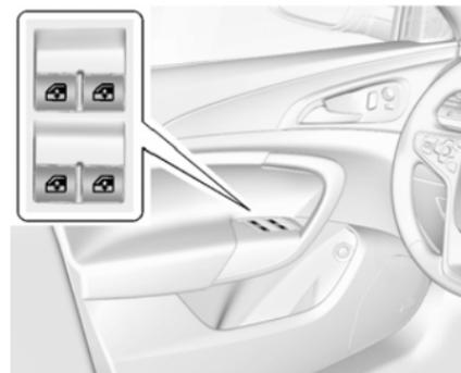
The power window switches are on the driver door. Each passenger door has a switch that controls only that window.
