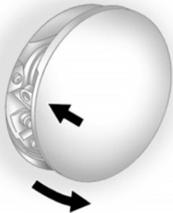
The fuel cap is behind a hinged fuel door on the passenger side of the vehicle. To open the fuel door, push and release the rearward center edge of the door.
