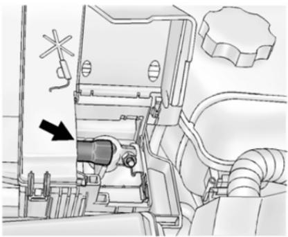
The vehicle has a remote positive (+) terminal under a trim cover. It is under the battery cover on the driver side of the engine compartment. See *Engine Compartment Overview on page 10-6*. You should always use this remote positive (+) terminal.
