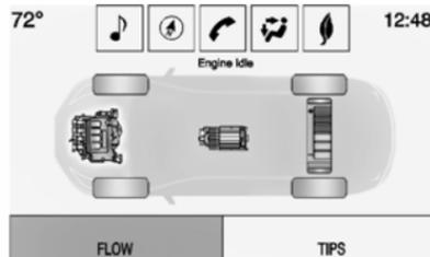
**Engine Idle** – Vehicle is stationary with engine active and no power is flowing to the wheels.
