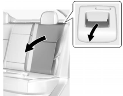
1. Pull on the lever on the top of the seatback to unlock it.
