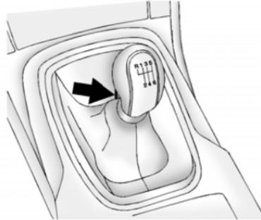
This is the shift pattern for the 6-speed manual transmission.
