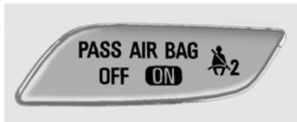
The words ON and OFF will be visible during the system check. When the system check is complete, either the word ON or the word OFF will be visible. See *Passenger Airbag Status Indicator on page 5-19*.
