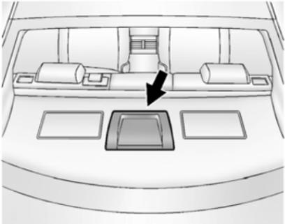
The eAssist system high voltage battery is cooled with air drawn from the vehicle interior. The cold air intake for the battery is behind the rear seat, on the filler panel. Do not cover the intake.
