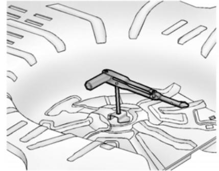
1. Turn the wrench counterclockwise to remove the fastener.
