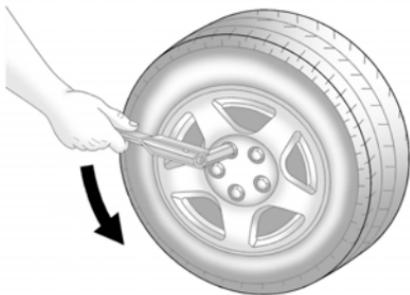
4. Turn the wheel wrench counterclockwise to loosen all the wheel nuts, but do not remove them yet.
