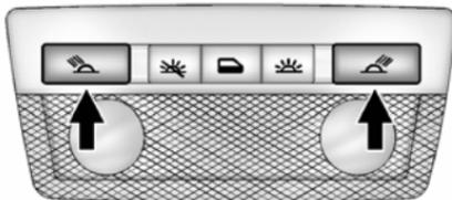
The front reading lamps are in the overhead console.
