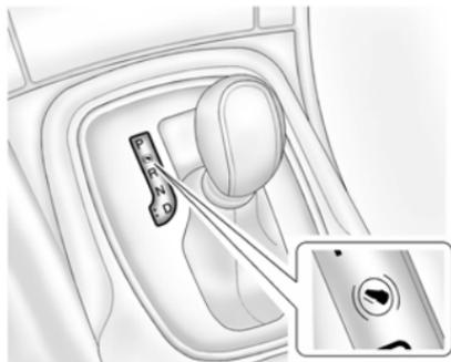
Without the brake pedal applied, the control indicator will be on.
