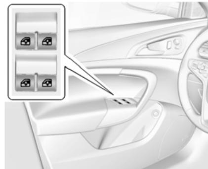
The power window switches on the driver door control all four windows. The passenger doors have a window switch for that window. Press the switch down to open the window. Pull the front of the switch up to close it.
