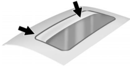
Dirt and debris may collect on the sunroof seal or in the track. This could cause an issue with sunroof operation or noise. It could also plug the water drainage system.
