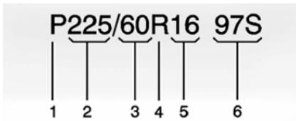
**(1) Passenger (P-Metric) Tire:** The United States version of a metric tire sizing system. The letter P as the first character in the tire size means a passenger
