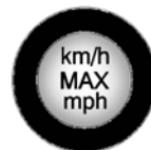
16. If the flat tire was able to inflate to the recommended inflation pressure, remove the maximum speed label from the tire sealant canister (5) and place it in a highly visible location. Do not exceed the speed on this label until the damaged tire is repaired or replaced.
