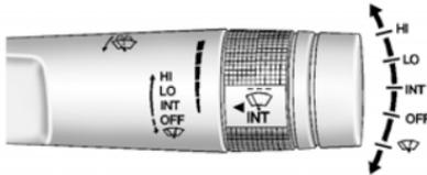
The windshield wiper/washer lever is on the right side of the steering column. With the ignition in ACC/ACCESSORY or ON/RUN, move the windshield wiper lever to select the wiper speed.
