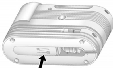
The tire sealant and compressor kit has an accessory adapter in a compartment on the bottom of its housing that may be used to inflate air mattresses, balls, etc.
