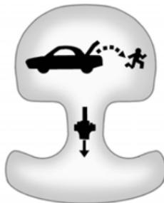
There is a glow-in-the-dark emergency trunk release handle on the trunk lid. This handle will glow following exposure to light. Pull the release handle to open the trunk from the inside.
