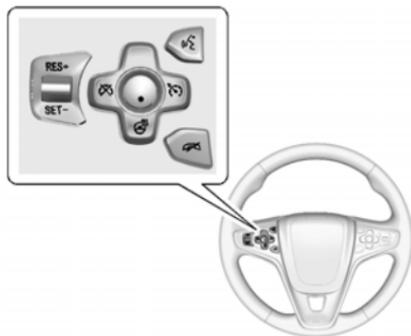
**⏻ (On/Off):** Press to turn cruise control on or off. A white indicator comes on in the instrument cluster when cruise is turned on.
