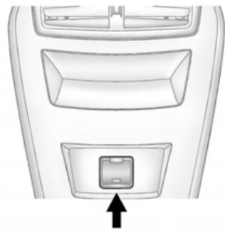
An indicator light on the outlet comes on when in use. The light comes on when the ignition is in ON/RUN, equipment requiring less than 150 watts is plugged into the outlet, and no system fault is detected.
