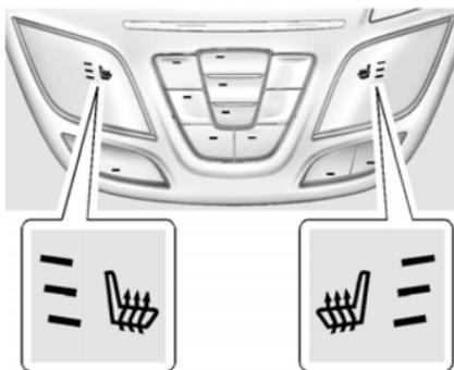
If equipped, the buttons are part of the climate control system on the center stack. To operate, the ignition and the climate control system must
