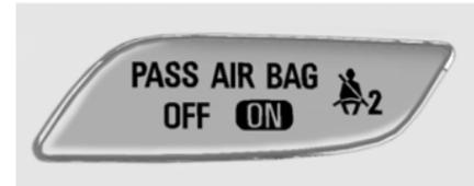
The passenger sensing system turns off the front outboard passenger frontal airbag under certain conditions. No other airbag is affected by the passenger sensing system.
