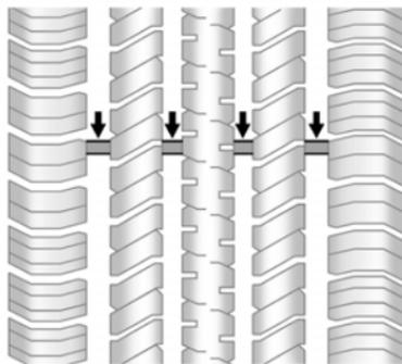
Treadwear indicators are one way to tell when it is time for new tires. Treadwear indicators appear when the tires have only 1.6 mm (1/16 in) or less of tread remaining. See *Tire Inspection* on page 10-54 and *Tire Rotation* on page 10-55.
