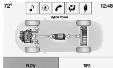
**Hybrid Power** – Both the engine and battery are active with energy flowing to the wheels.
