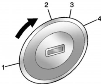
The ignition switch has four different positions.
