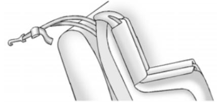
If the position you are using does not have a headrest or head restraint, or the headrest or head restraint has been removed, and you are using a dual tether, route the tether over the seatback.
