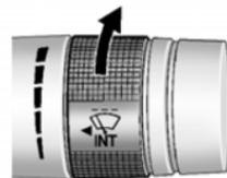
**INT:** Move the lever up to INT for intermittent wipes, then turn the
