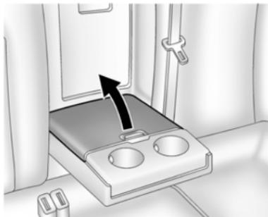
Pull down the armrest. Press the button to lift the cover. Close the cover before folding the armrest up.
