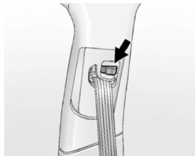
Press down on the release button and move the height adjuster to the desired position. The adjuster can be moved up by pushing the slide/trim up. After the adjuster is set to
