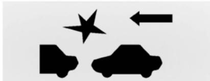
When your vehicle approaches another detected vehicle too rapidly, the red FCA display will come on. Also, eight rapid high-pitched beeps will sound from the front. When this Collision Alert occurs, the brake system may prepare for driver braking to occur more rapidly which can cause a brief, mild deceleration. Continue to apply the brake pedal as needed. Cruise control may be disengaged when the Collision Alert occurs.
