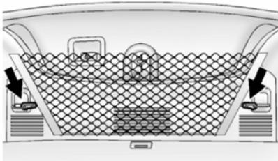
If equipped, the convenience net is in the trunk and can be used to store small loads. The net should not be used to store heavy loads. Attach the loops on each side of the net to the hooks located on the sides of the trunk.
