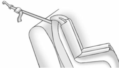
If the position you are using does not have a headrest or head restraint, or the headrest or head restraint has been removed, and you are using a single tether, route the tether over the seatback.
