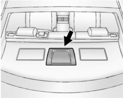
The cold air intake for the battery is located behind the rear seat, on the filler panel. Do not cover the intake. See *Battery* on page 10-26.
