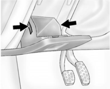
The instrument panel fuse block is located in the instrument panel, on the driver side of the vehicle.
