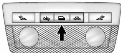
The interior lamps control in the overhead console controls both the front and rear interior lamps.
