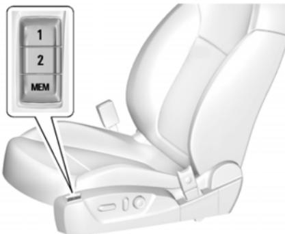
If equipped, the MEM, "1," and "2" buttons on the outboard side of the driver seat are used to manually save and recall the driver seat and outside mirror positions.
