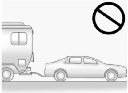
The vehicle was not designed to be towed from the rear with all four wheels on the ground.
