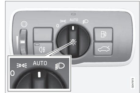
Headlight switch in the AUTO position
