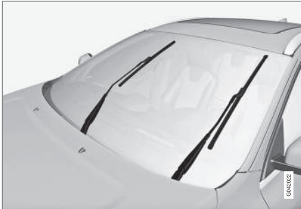
Wiper blades in service position
