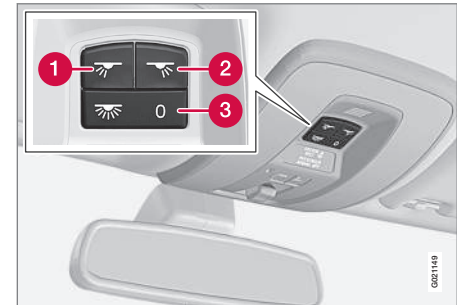
Light switches, front roof lighting
