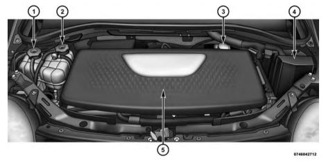
1 — Battery Thermal Coolant Reservoir
