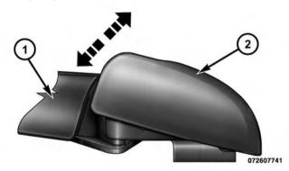
**NOTE:** The rear wiper arm cannot be raised fully upward unless the pivot cap is raised first.
