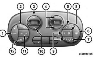
Automatic Temperature Controls 1. AUTO Temperature Control (ATC) Button
