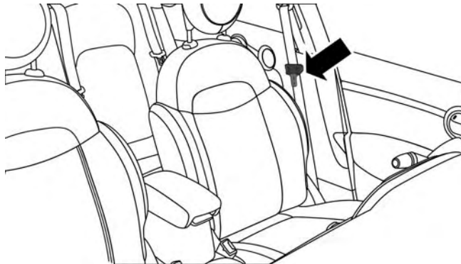
Pulling Out The Latch Plate
