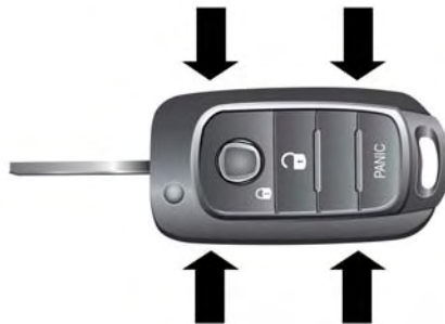
Integrated Vehicle Key Battery Removal
