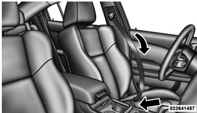
Pulling Out The Latch Plate
