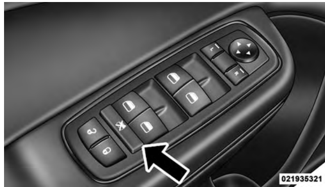
Window Lockout Switch
