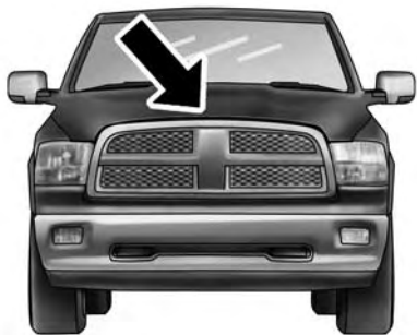
Safety Latch Location (1500 Series Shown)
