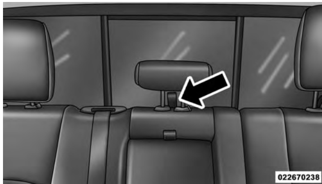
Tether Strap Loop With Center Head Restraint In Raised Position
