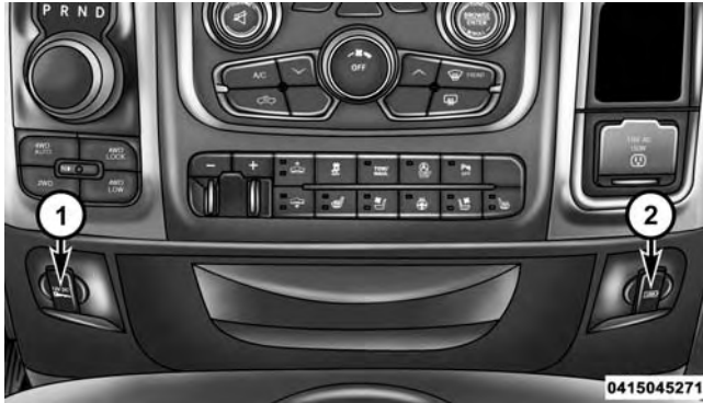
Power Outlets — Center Stack
