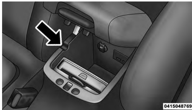
Center Console USB/AUX Connector Port Cable Routing
